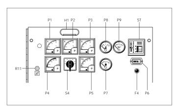
The control and indicator panel is located behind a door in the side panel. The hinged door is partly transparent and allows easy access to the parts mounted behind it. The panel light (H1) lights up as soon as the starter switch is turned into position 1 or the remote start/stop switch is put in position start, indicating that the fuel solenoid is energised.
