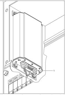
When starting up the generator, the green Power Led (1) of the Cosmos module will light up when the installation has been carried out correctly.
