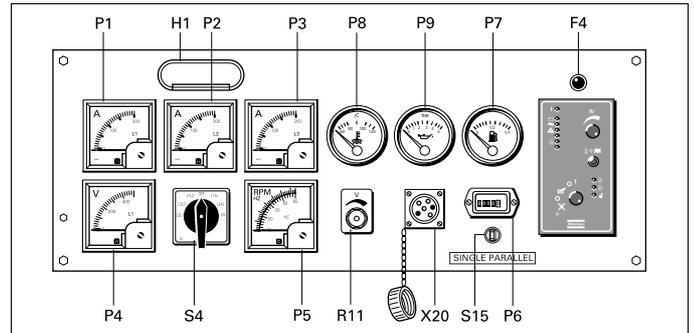
The control and indicator panel is located behind a door in the side panel. The hinged door is partly transparent and allows easy access to the parts mounted behind it. Panel light H1 lights up as soon as the starter switch is turned into position I or the remote start/stop switch is put in position start, indicating that the fuel solenoid is energized.
