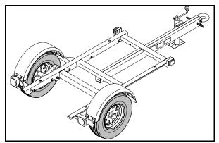
The fixed towbar trailer is equipped with a torsion axle, standard pintle towing eye, tongue mounted jack and trailer lighting system.
