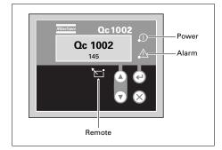
Power Remote Green LED indicates that the unit is powered up.
