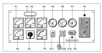
The control and indicator panel is located behind a door in the side panel. The hinged door is partly transparent and allows easy access to the parts mounted behind it. Panel light H1 lights up as soon as the starter switch is turned into position I or the remote start/stop switch is put in position start, indicating that the fuel solenoid is energized.
