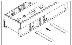
The earthing rod, connected to the generator's earth terminal is located at the bottom of the frame on the outside.
