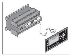
The Qc4002<sup>TM</sup> module is located inside the control panel, and communicates with a display unit, located in front of the control panel. This control module will carry out all necessary tasks to control and protect a generator, regardless of the use of the generator.
