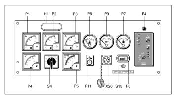
The control and indicator panel is located behind a door in the side panel. The hinged door is partly transparent and allows easy access to the parts mounted behind it. Panel light H1 lights up as soon as the starter switch is turned into position I or the remote start/stop switch is put in position start, indicating that the fuel solenoid is energized.
