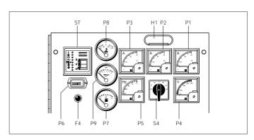
The control and indicator panel is located behind a door in the side panel. The hinged door is partly transparent and allows easy access to the parts mounted behind it. The panel light (H1) lights up as soon as the starter switch is turned into position ① or the remote start/stop switch is put in position start, indicating that the fuel solenoid is energised.
