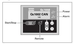
Power Green LED indicates that the unit is powered
