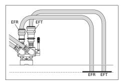
EFT EFR External fuel tank connection
