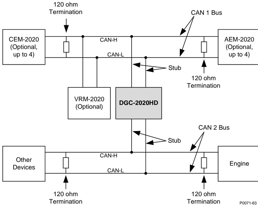
Figure 27. CAN Interface with Other Devices Providing One End of the Bus.
