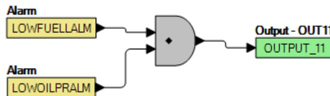
Figure 42. Example 2 – AND Gate Connections
