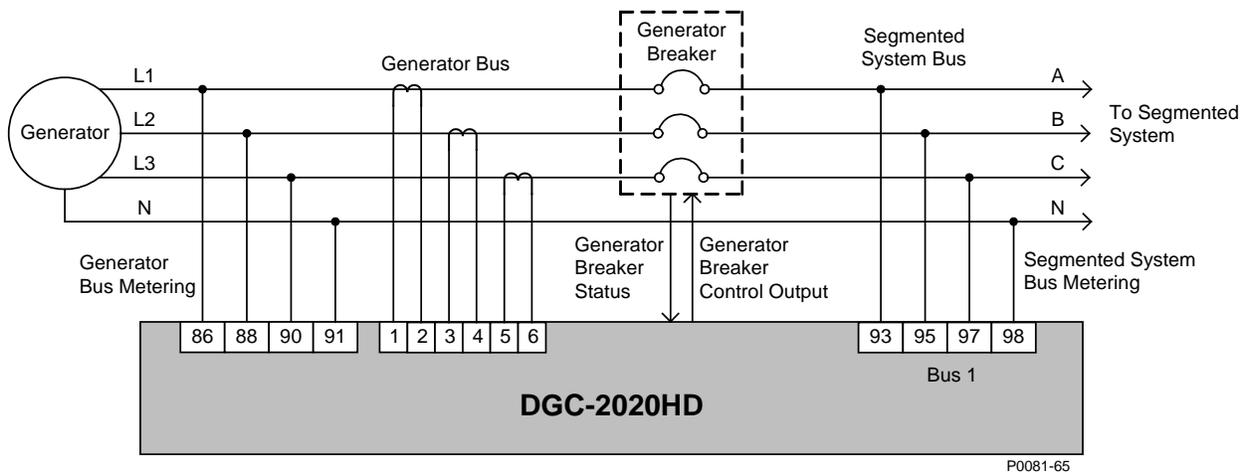
**Figure 18. Generator Breaker Control to Segmented System Connections**
