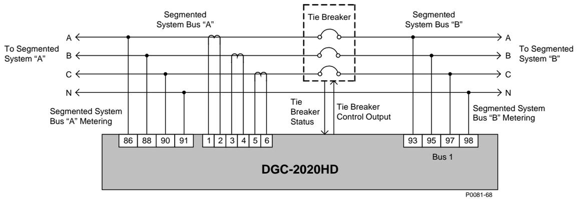
**Figure 21. Tie Breaker Control Connections**
