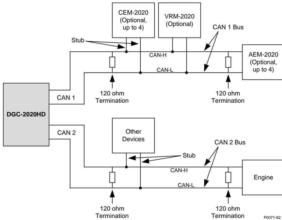
**Figure 37. CAN Interface with DGC-2020HD Providing One End of the Bus**
