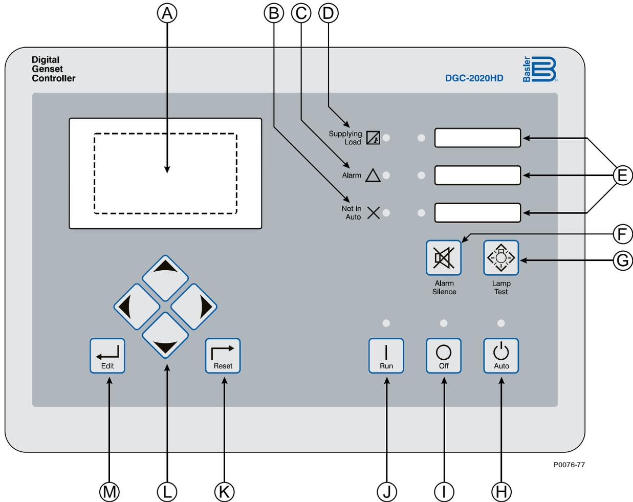
Figure 44. Front-Panel Controls and Indicators
