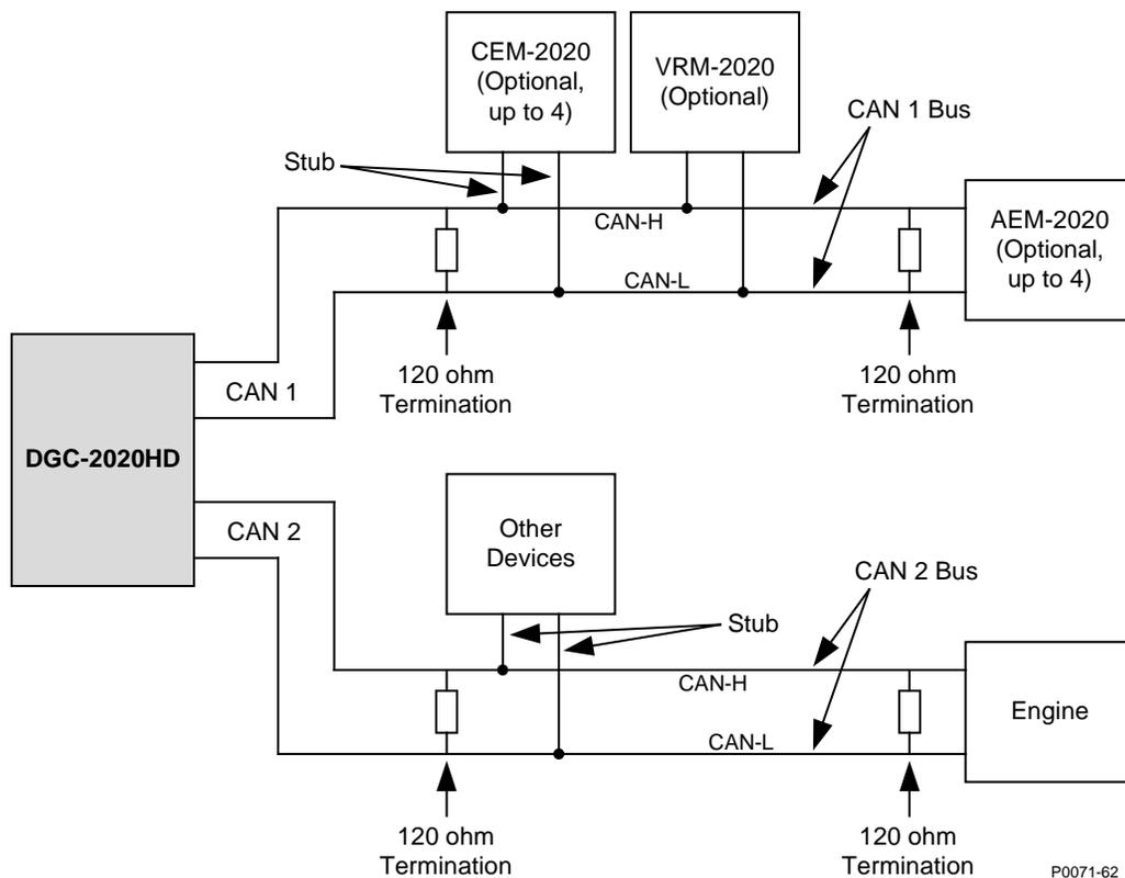
Figure 26. CAN Interface with DGC-2020HD Providing One End of the Bus
