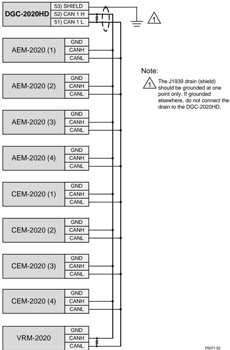
Figure 28. DGC-2020HD Expansion Module CAN Connections
