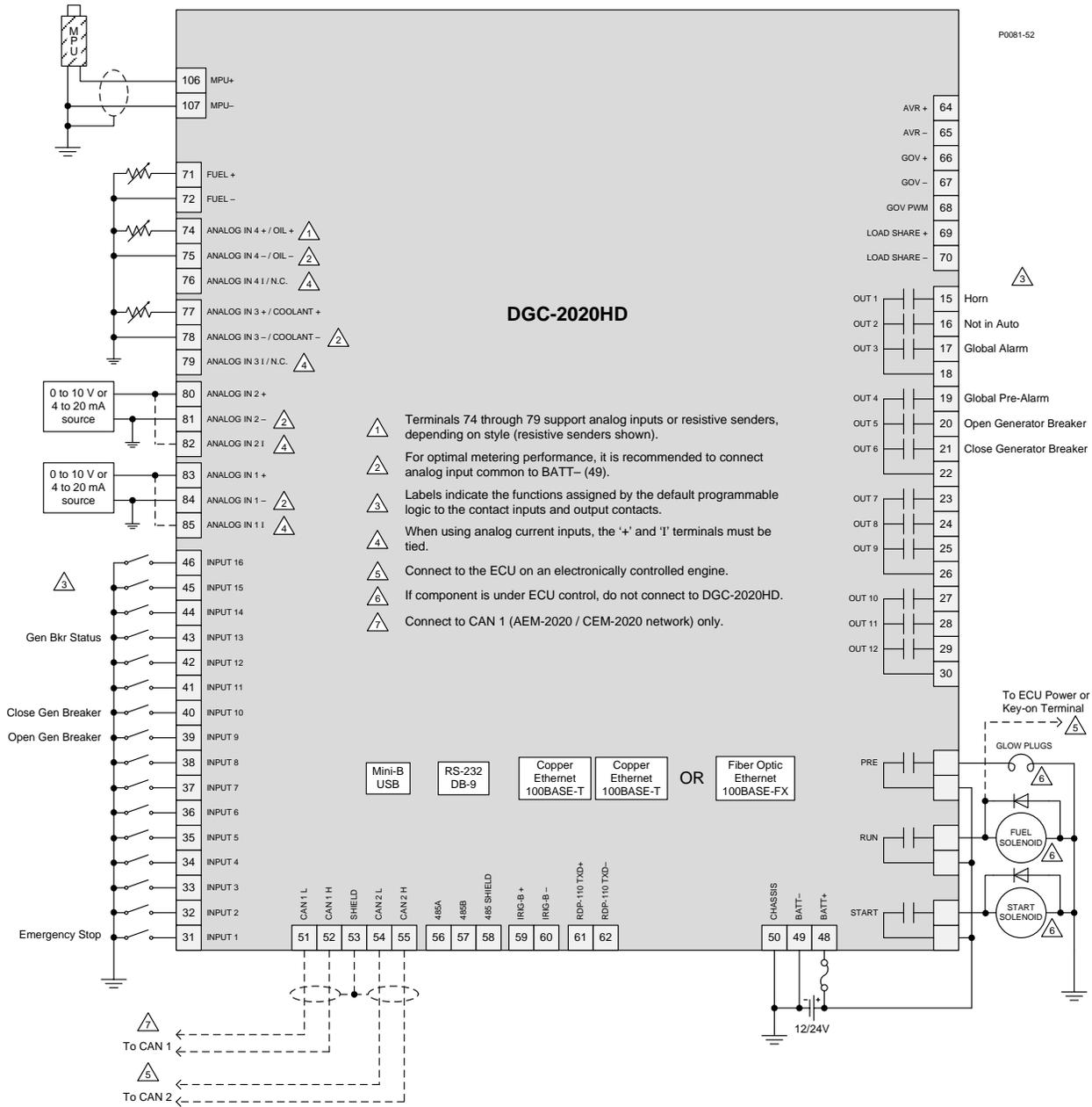
**Figure 5. Connections for Communication, Senders, Contact Inputs and Outputs, and Control Power**
