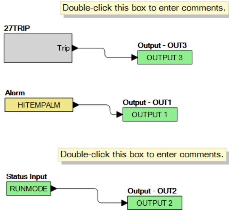
Figure 43. Example 3 – Multiple Logic Connections
