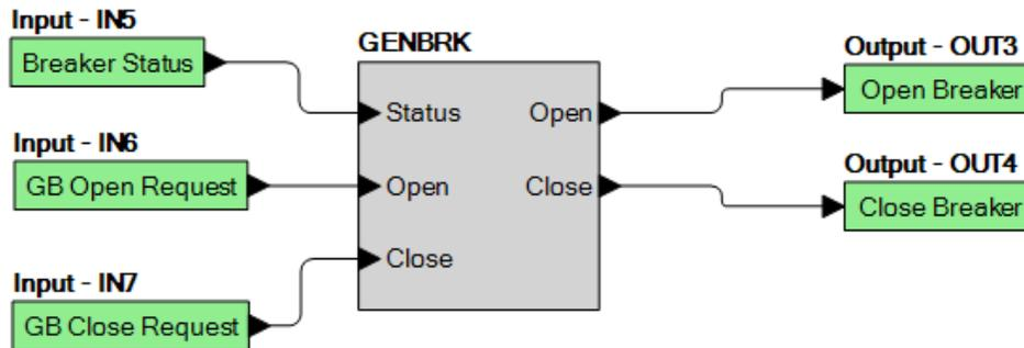
Figure 41. Example 1 – GENBRK Logic Block Connections
