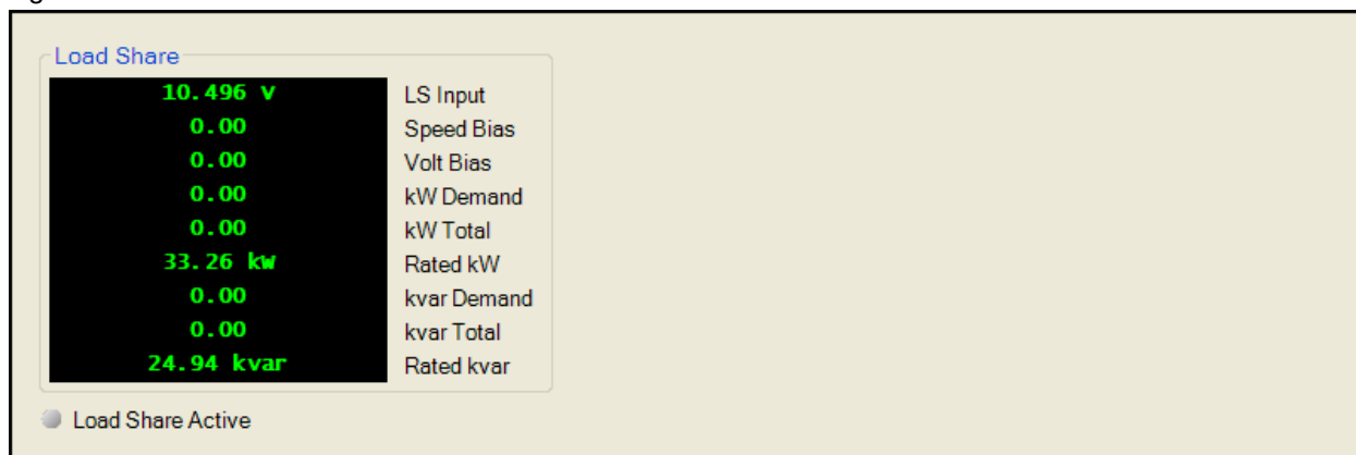
Figure 122. Metering Explorer, Diagnostics, Load Share Screen
