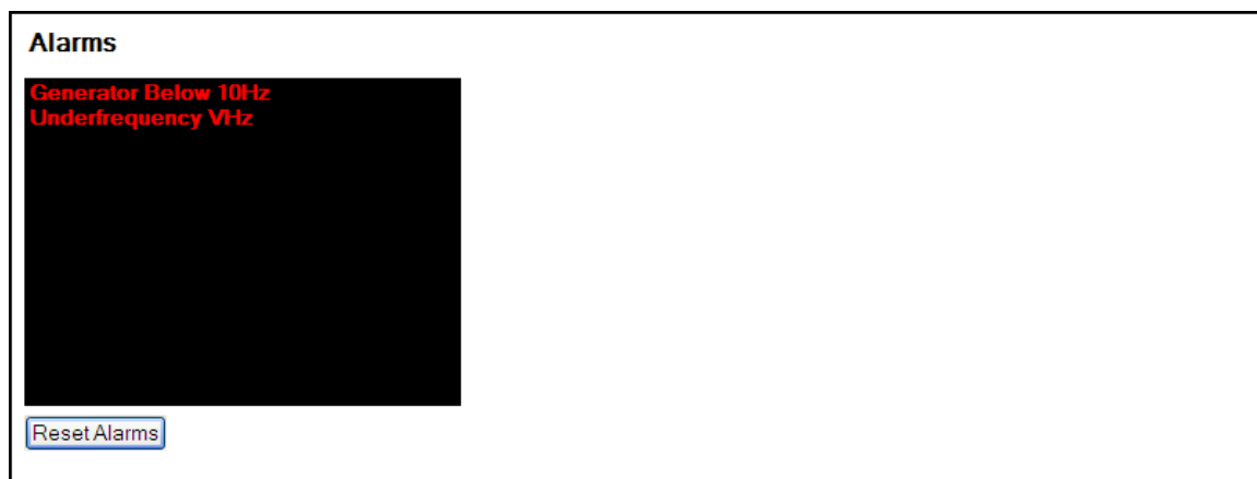
Figure 96. DECS-250 Alarm Annunciation and Reset Screen
