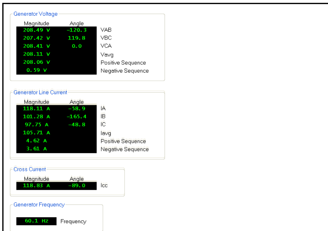
Figure 79. Generator Primary-Values Metering
