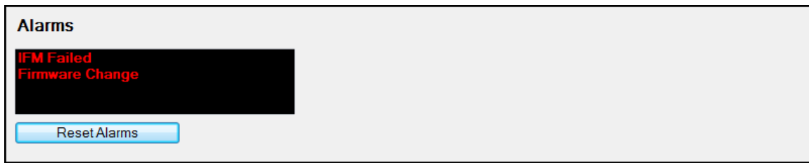
Figure 79. DECS-250E Alarm Annunciation and Reset Screen
