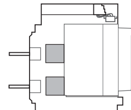
Masterpact Circuit Breaker Equipped for Remote ON/OFF Function Cluster shield is not shown
