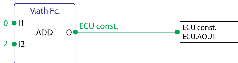
Image 2.3 PLC constant for ECU control
