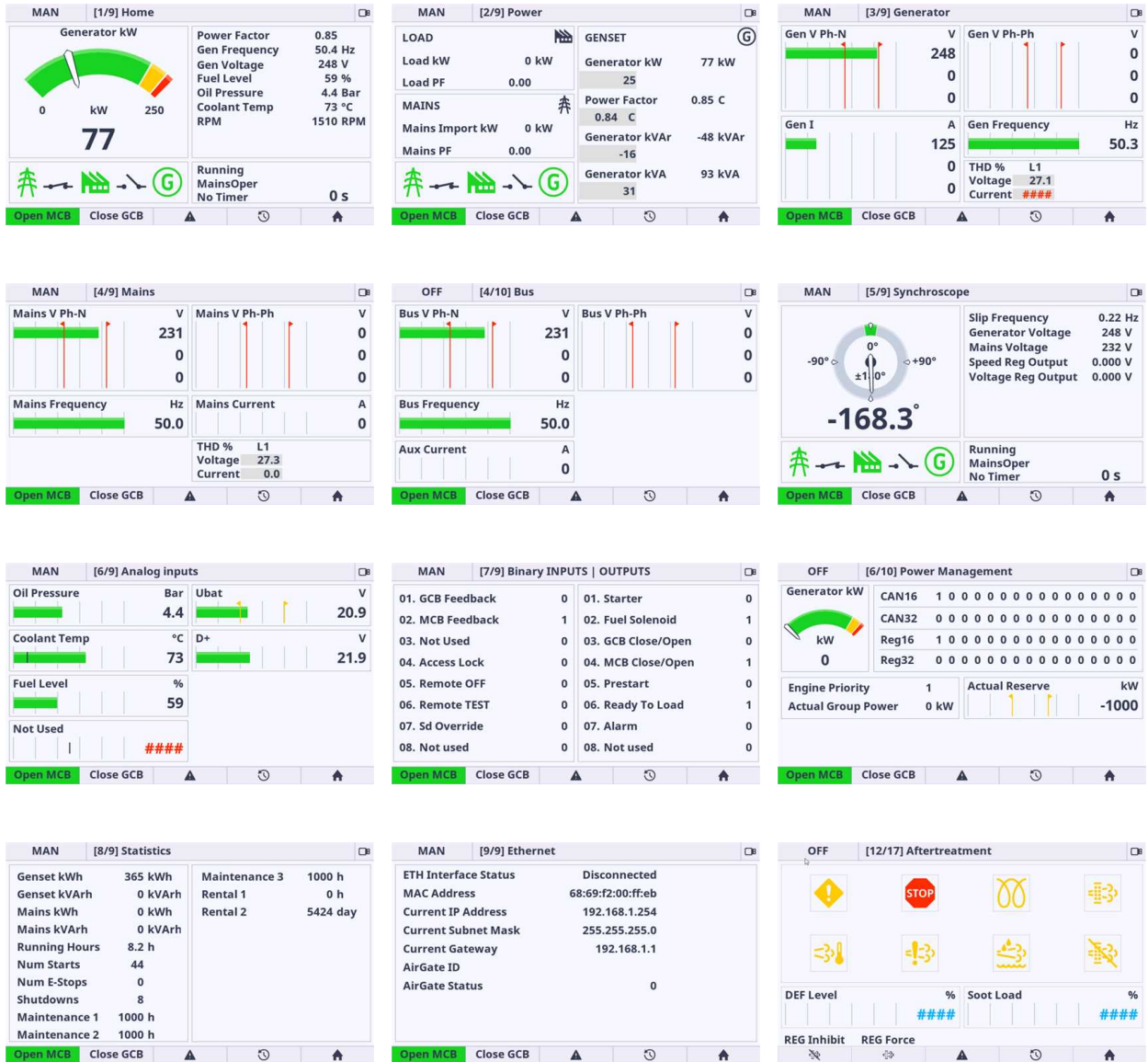
Image 2.1 : IntelliGen 500 metering screens overview
