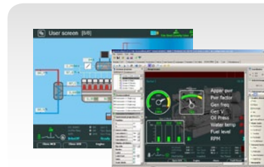
ScreenEditor PC tool, which allows you to personalise the interface on your InteliVision 5 and InteliVision 8 colour displays, part of GenConfig and DriveConfig.
