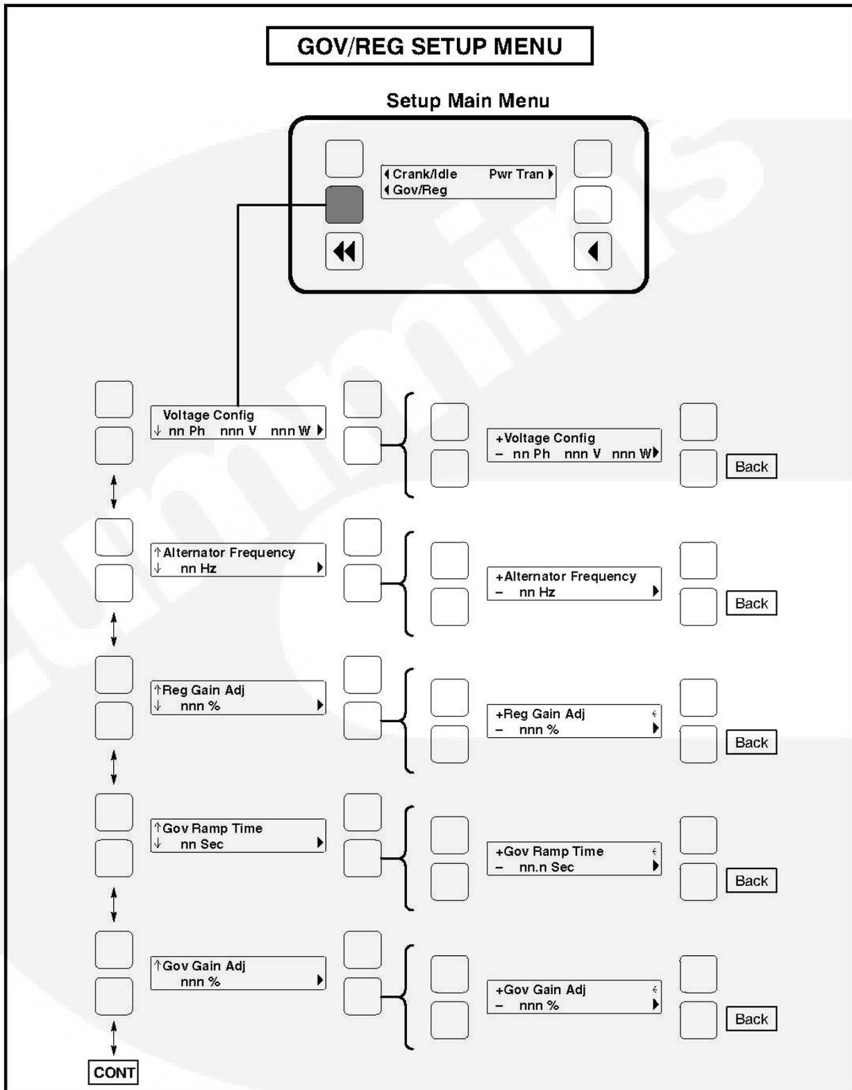
FIGURE 28. GOVERNOR/REGULATOR SETUP MENU (1 OF 2)
