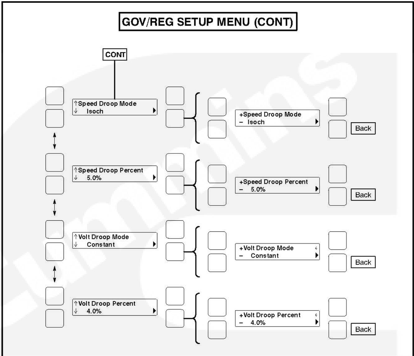
**FIGURE 29. GOVERNOR/REGULATOR SETUP MENU (2 OF 2)**
