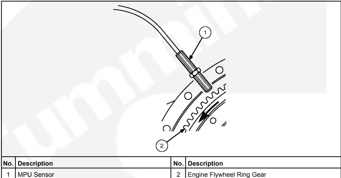
FIGURE 32. MPU SENSOR
