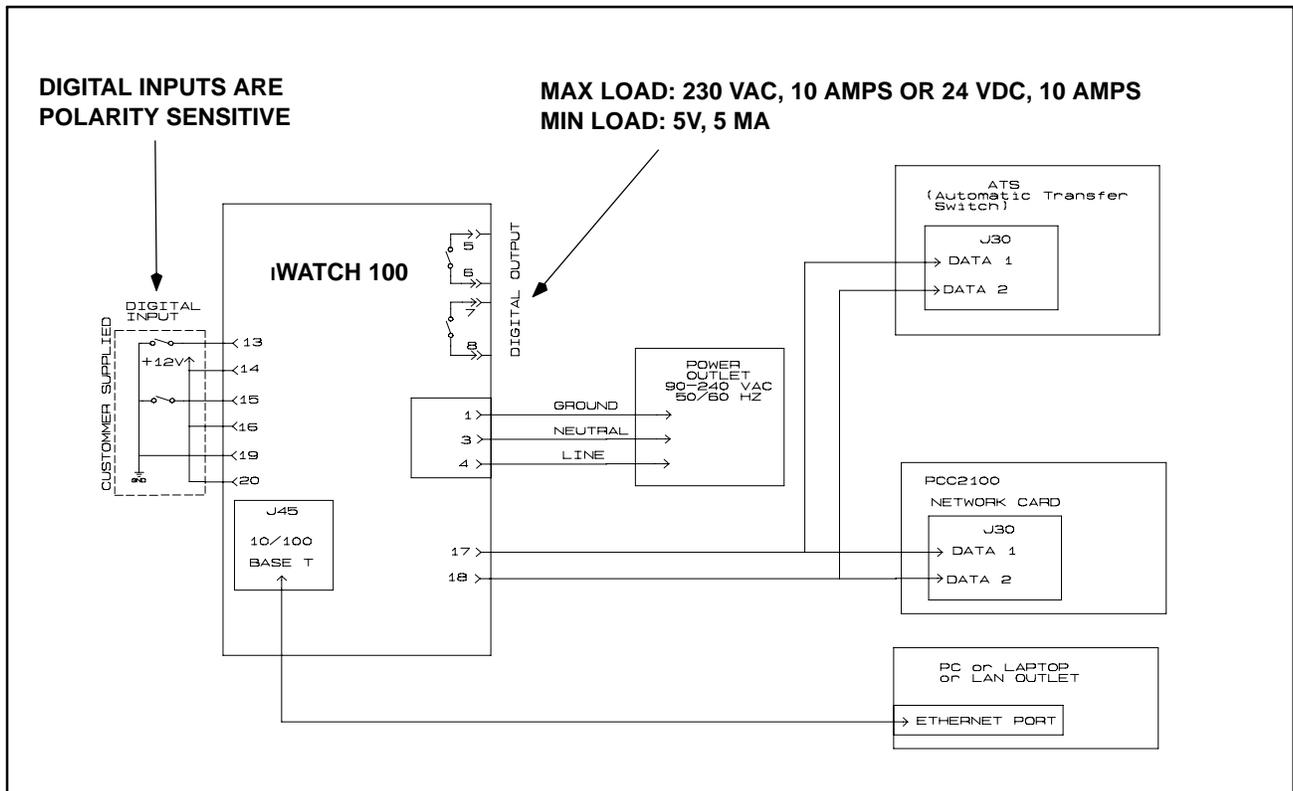
**FIGURE 3-9. POWERCOMMAND iWATCH 100 WITH POWERCOMMAND 2100 CONTROL**
