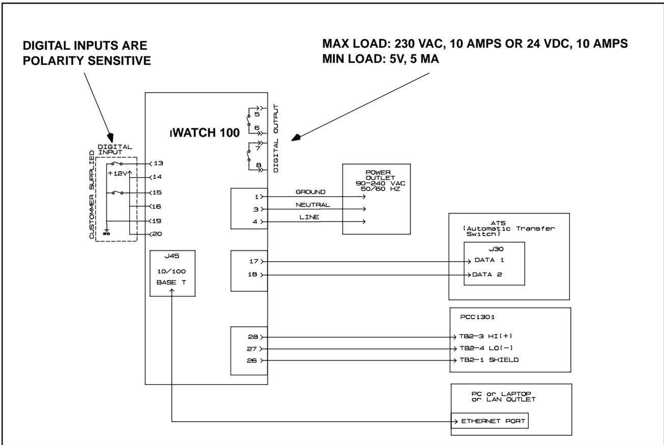
**FIGURE 3-11. POWERCOMMAND iWATCH 100 WITH POWERCOMMAND 1.X, 2.X, 3.X CONTROL**
