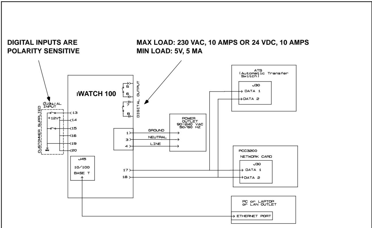
**FIGURE 3-10. POWERCOMMAND iWATCH 100 WITH POWERCOMMAND 3200 CONTROL**
