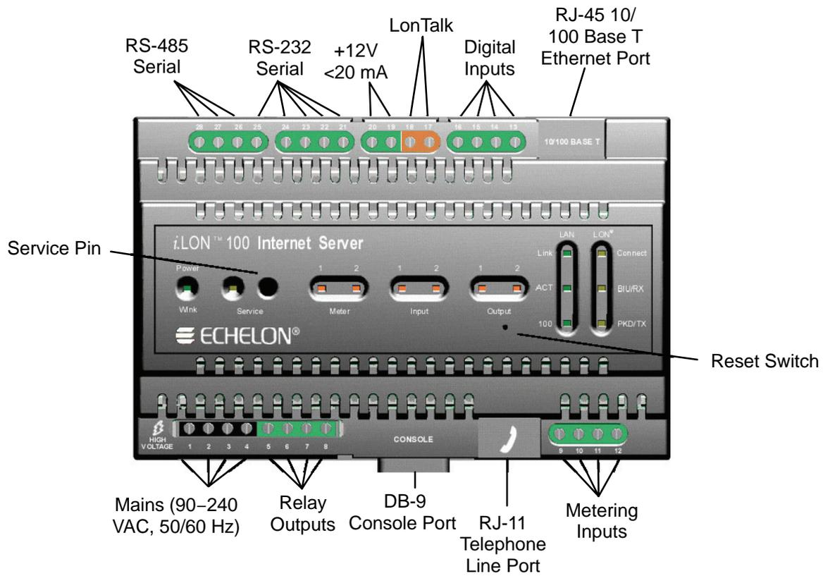
FIGURE 3-3. *i*.LON 100 SERVER DATA, CONSOLE, AND TELEPHONE CONNECTIONS
