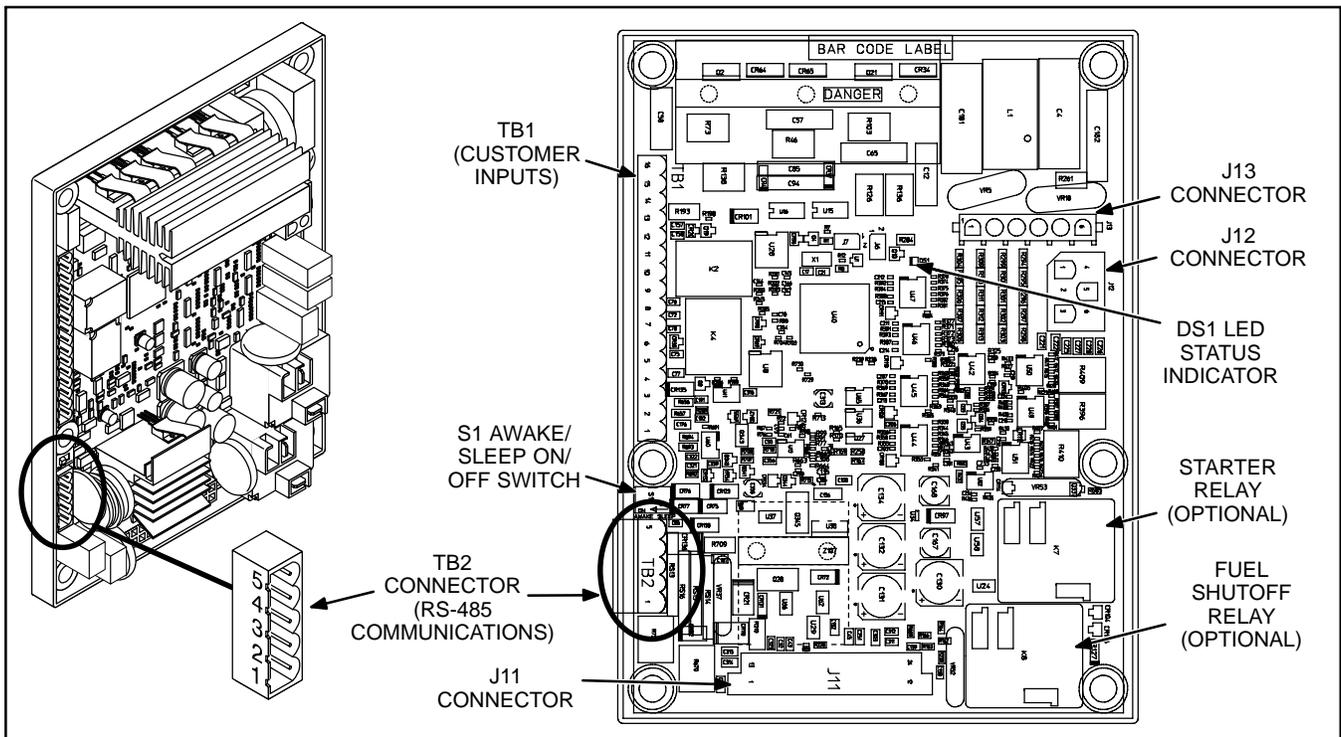
FIGURE 3-5. PCC1301 CONTROL BOARD WITH RS-485 COMMUNICATIONS PORT
