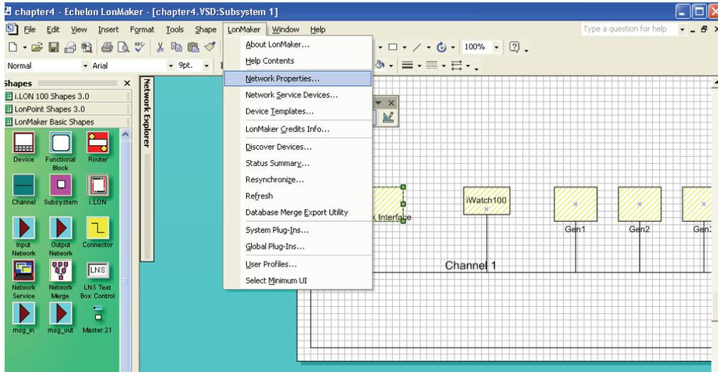
**FIGURE 4-25. CONNECTING TO THE NETWORK INTERFACE**
