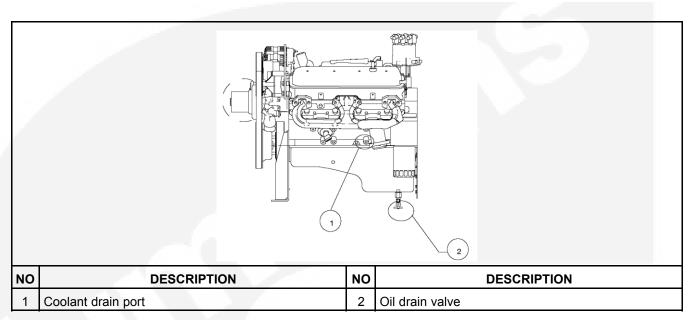
FIGURE 22. DRAIN PORTS LOCATIONS FOR ENGINE OIL AND COOLANT
