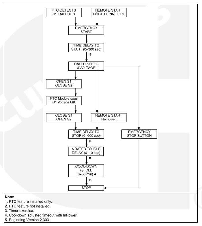
FIGURE 15. STARTING FROM A REMOTE LOCATION (REMOTE START SIGNAL) - AUTO MODE
