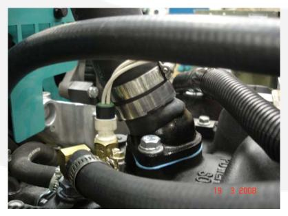
FIGURE 19. LP VAPORIZER ON ENGINE (IF USED)
