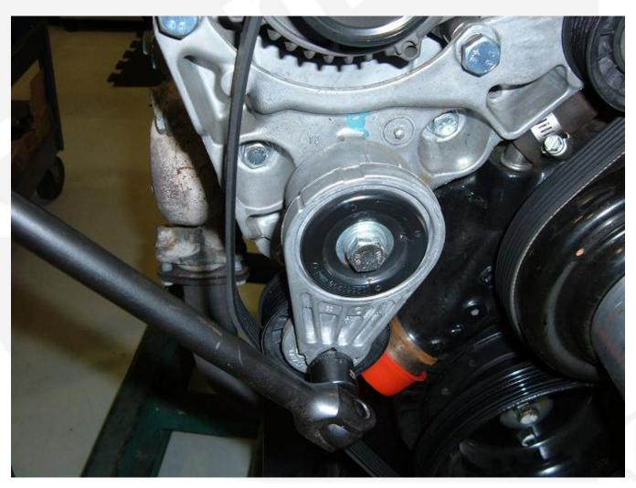
FIGURE 25. BELT REPLACEMENT WITH RATCHET INSERTED IN TENSIONER
