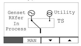
FIGURE 20. BUILDING LOAD TRANSFER IN PROCESS
