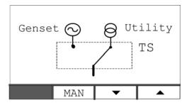
FIGURE 21. UTILITY POWERING BUILDING LOAD
