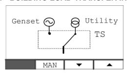
FIGURE 35. UTILITY POWERING BUILDING LOAD
