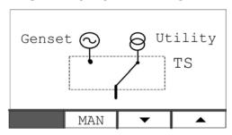
FIGURE 28. UTILITY POWERING BUILDING LOAD
