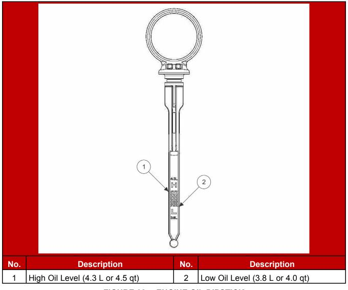
FIGURE 38. ENGINE OIL DIPSTICK
