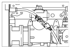
FIGURE 41. CHECK HARNESS CONNECTIONS
