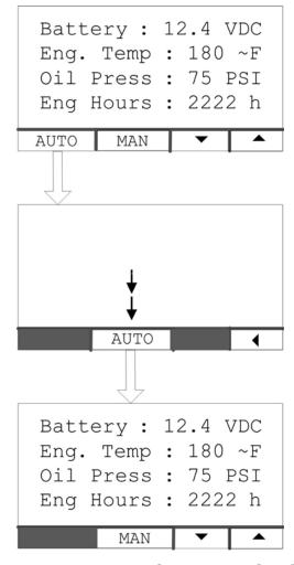
FIGURE 29. HMI211 SET IN AUTO MODE
