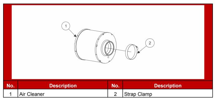
FIGURE 39. EXAMPLE OF NORMAL DUTY AIR CLEANER
