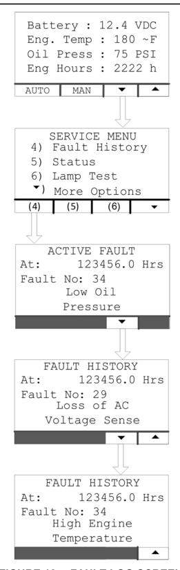
FIGURE 12. FAULT LOG SCREEN
