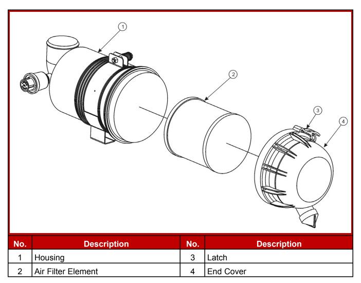
FIGURE 40. EXAMPLE OF HEAVY DUTY AIR CLEANER
