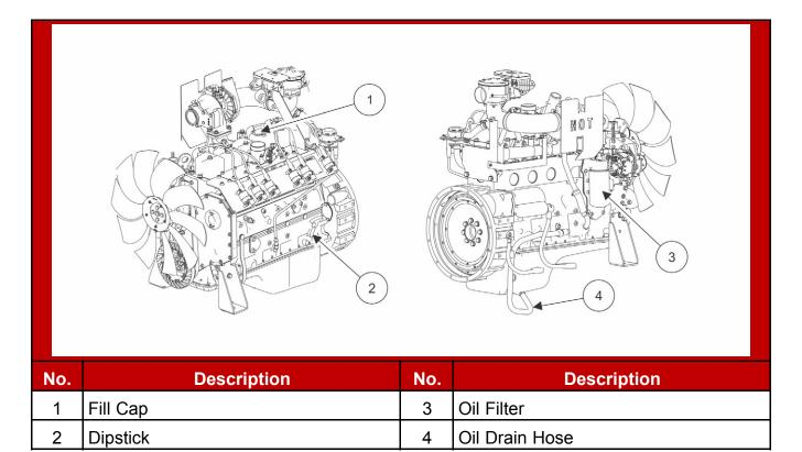
FIGURE 37. ENGINE OIL COMPONENTS
