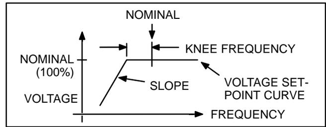
FIGURE 6-5. KNEE FREQUENCY AND SLOPE
