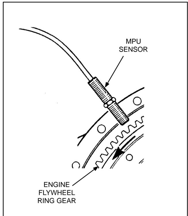
**FIGURE 6-20. MPU SENSOR**
