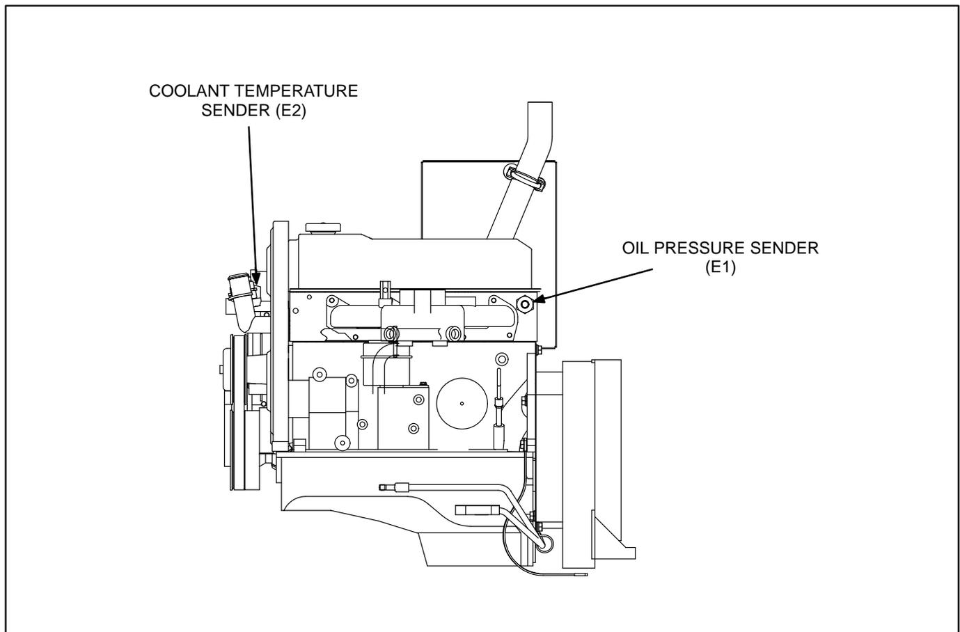
FIGURE 6-19. FOUR CYLINDER ENGINE SENSOR LOCATIONS
