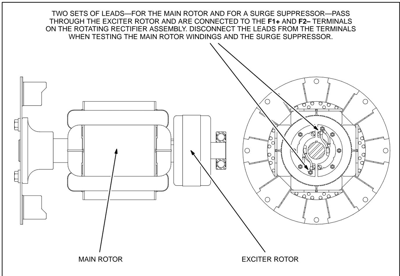
FIGURE 7-4. TESTING THE MAIN ROTOR
