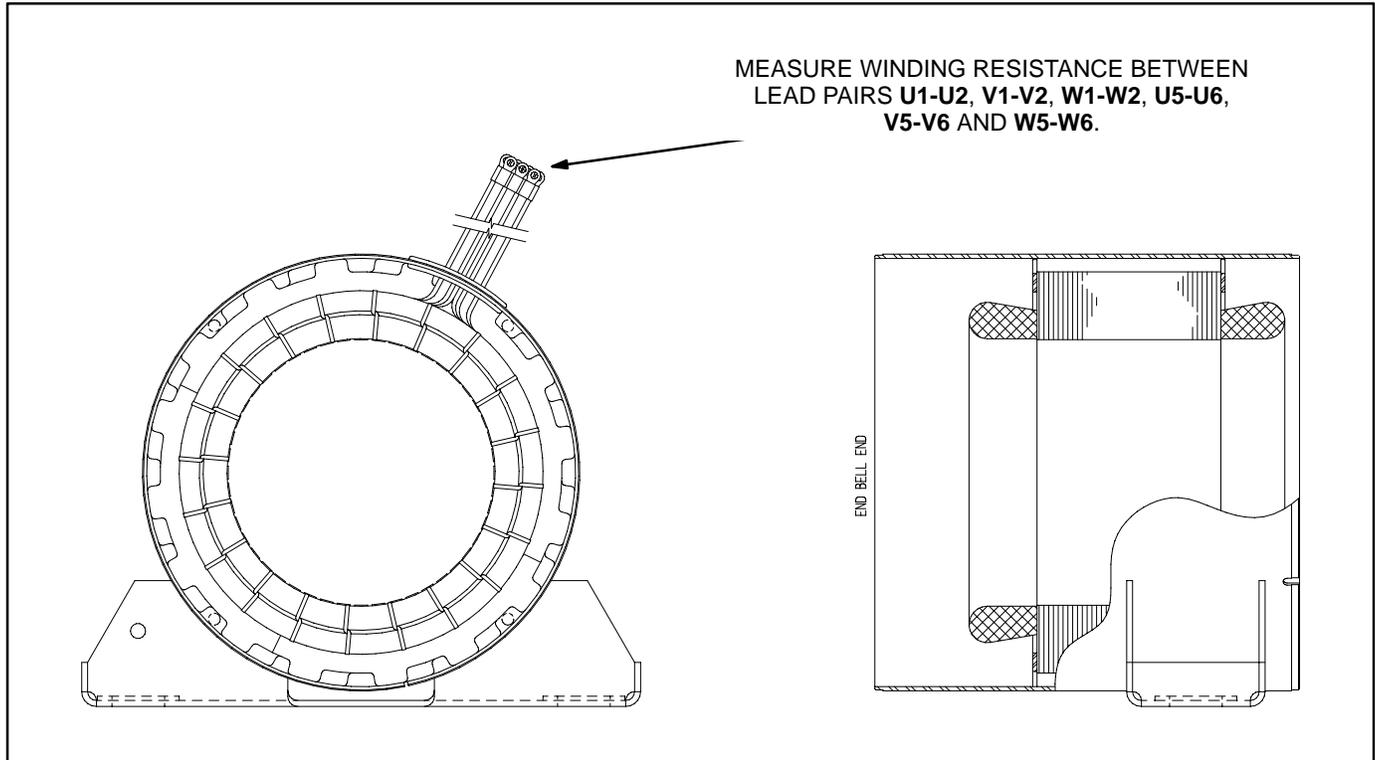
**FIGURE 7-5. TESTING THE MAIN STATOR WINDINGS**
