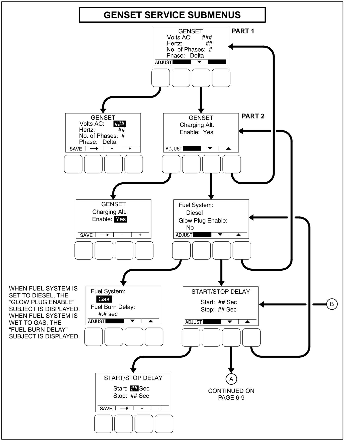
FIGURE 6-4. GENSET SERVICE SUBMENUS (SHEET 1 OF 3)
