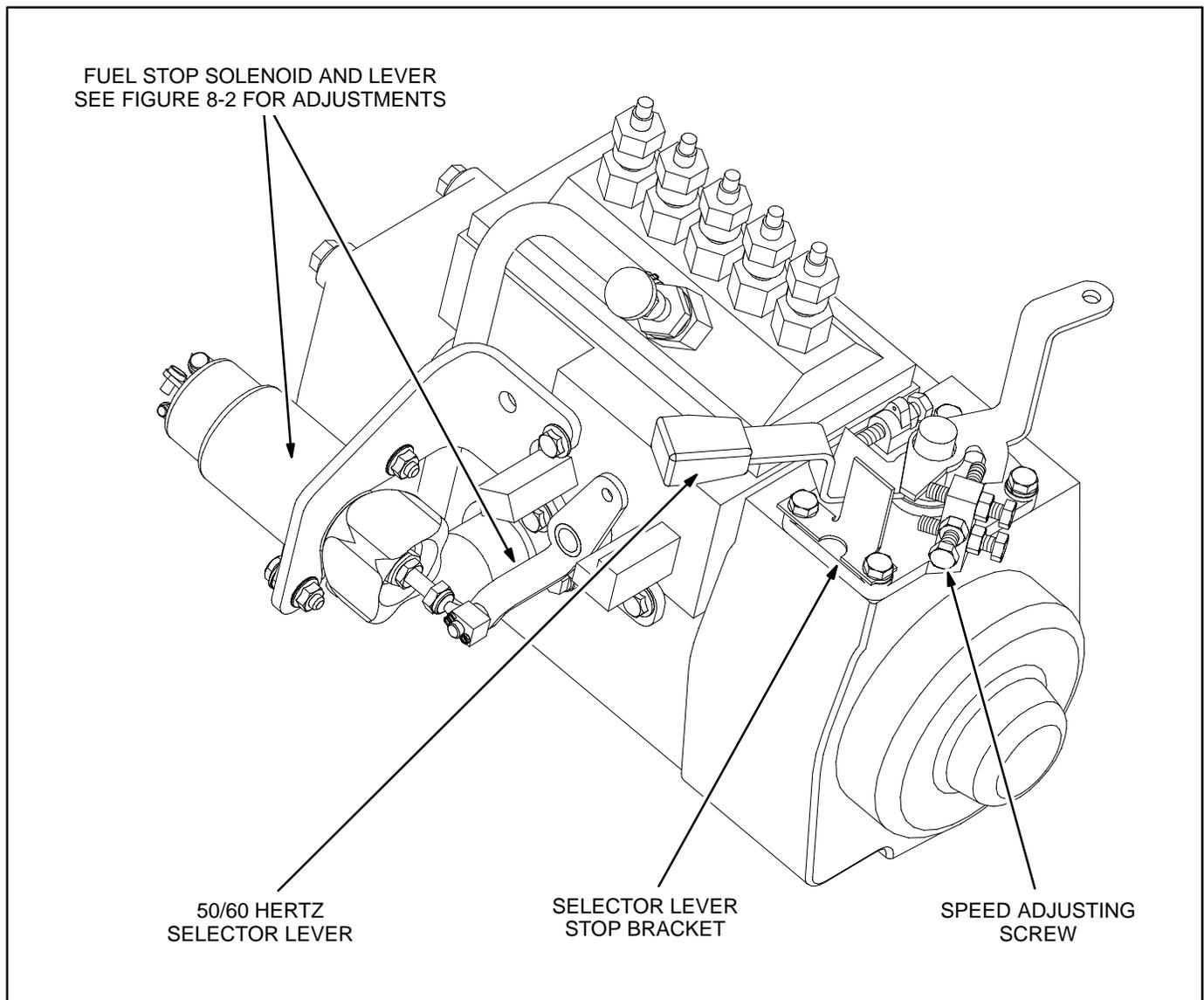
FIGURE 8-1. GOVERNOR AND FUEL INJECTION UNIT
