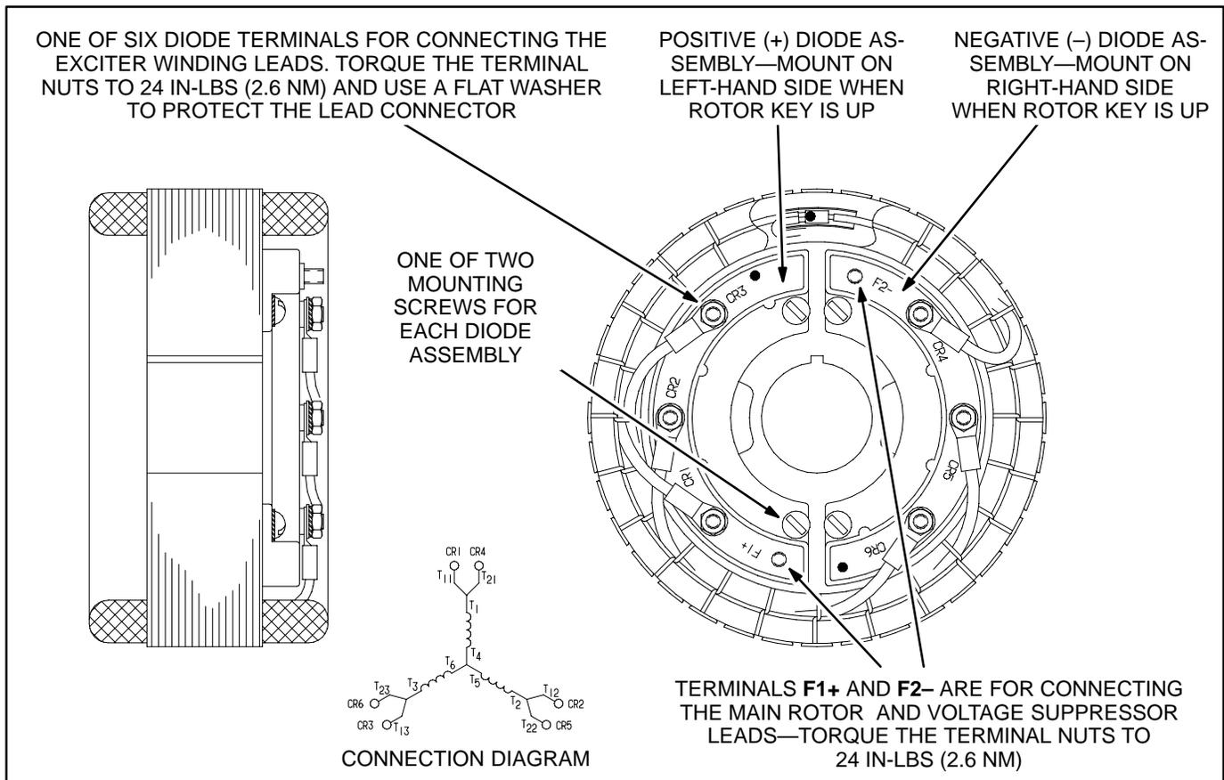
FIGURE 7-3 TESTING THE ROTATING RECTIFIER ASSEMBLY
