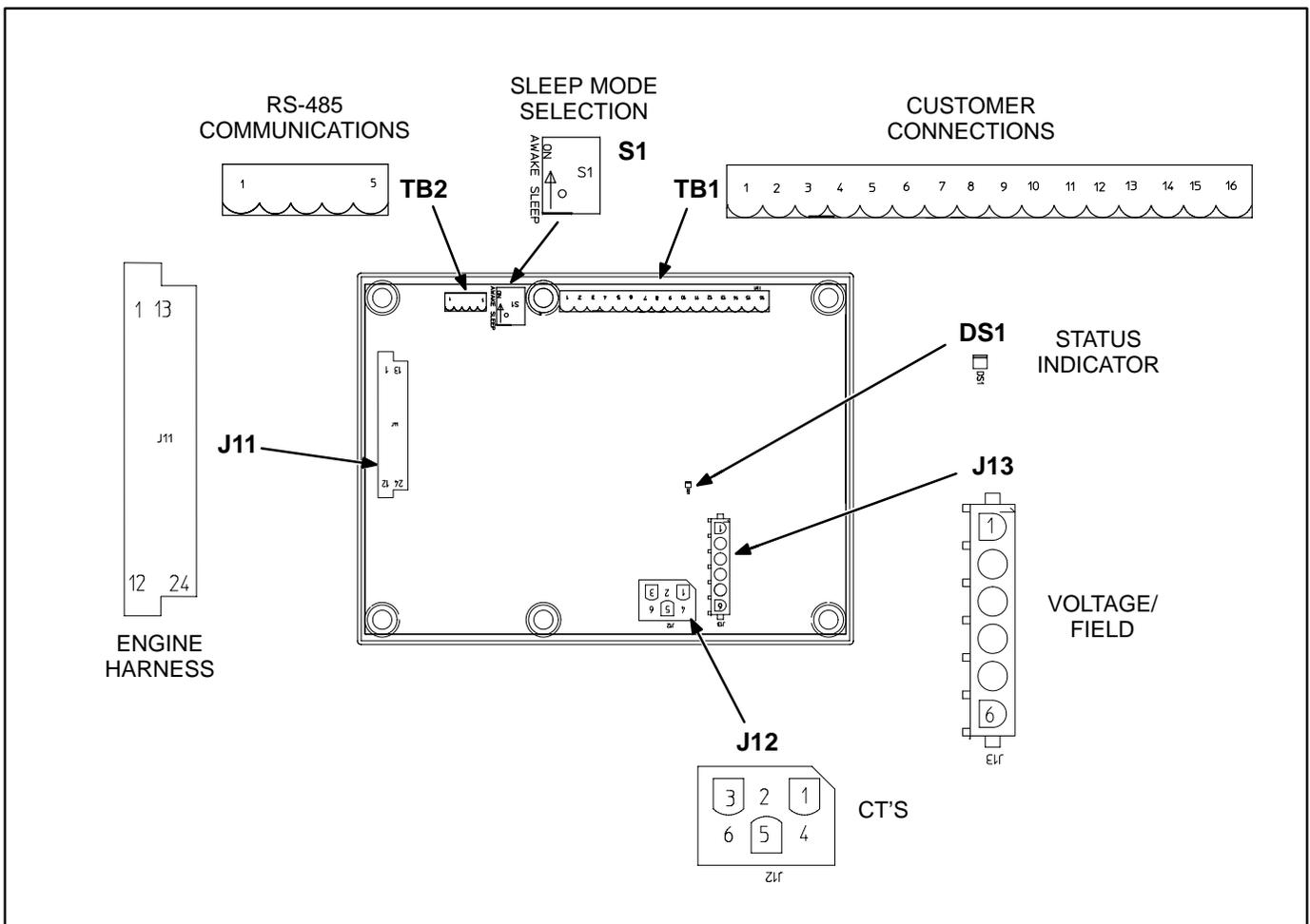
FIGURE 4-4. BASE BOARD CONNECTOR/TERMINAL PIN LOCATIONS
