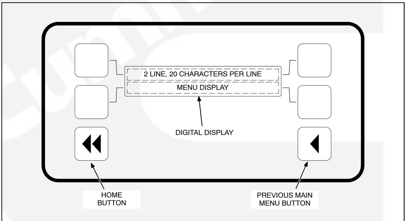
**FIGURE 2-2. DIGITAL DISPLAY AND MENU SELECTION BUTTONS**
