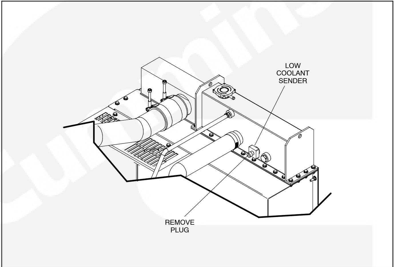
FIGURE 5-10. LOW ENGINE COOLANT SENSOR
