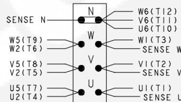
NOTE: FOR SHUNT OPERATION, CONNECT AC HARNESS LEADS:
