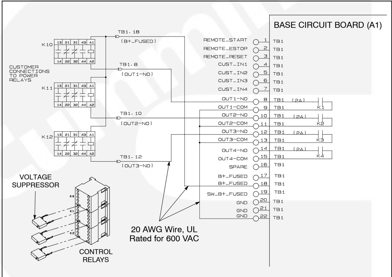
FIGURE 5-8. OPTIONAL CONTROL RELAYS (K10, K11, K12)
