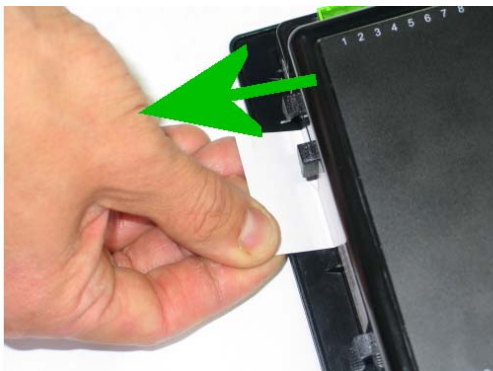
Removal and insertion of the LED text insert card
