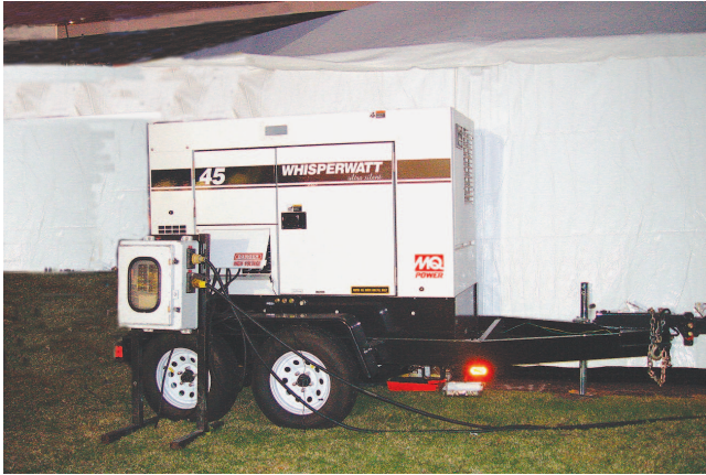
Exhibit 2. A Trailer (Vehicle) Mounted Portable Generator (Not Permitted as an EPS). (Courtesy of the International Association of Electrical Inspectors)
