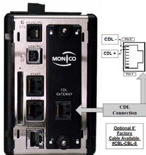
Figure 3.1 CDL Connection Pin #7=CDL (+); Pin#8=CDL (-)
