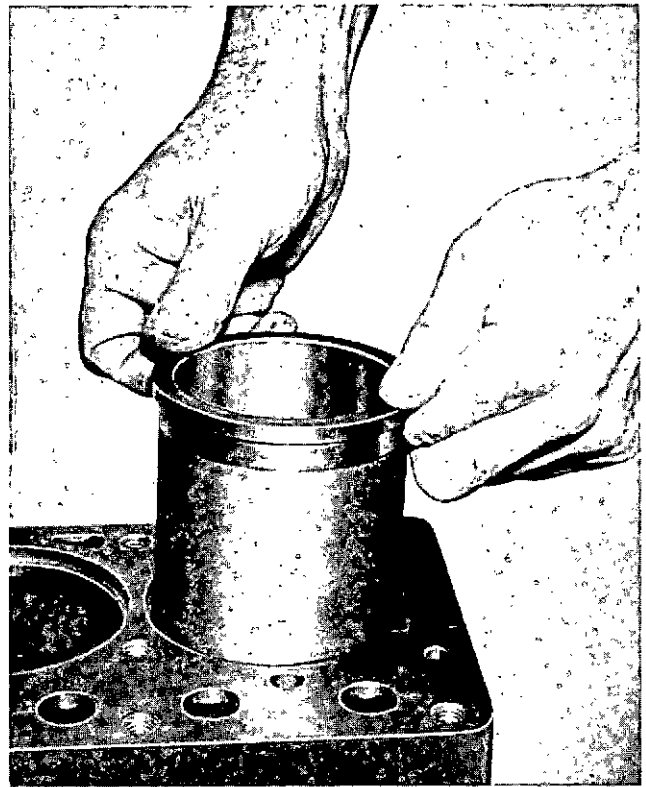
Figure 155 — Installing Sleeve in Block
