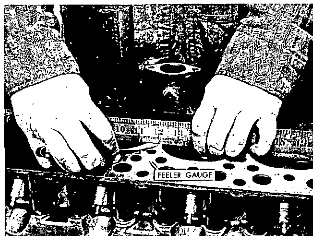
Figure 135 Checking Cylinder Head Flatness
