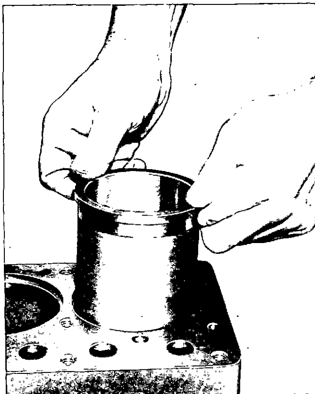
Figure 170—Installing Sleeve in Block
