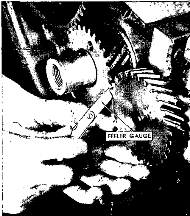
Figure 210—Checking Backlash Between Crank Gear and Oil Pump Drive Gear
