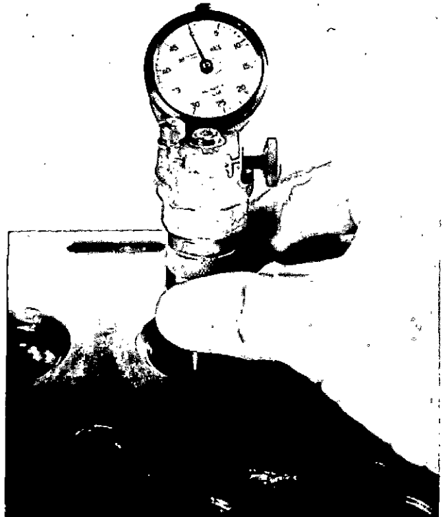
Figure 145—Checking Intake Valve Seat Run-Out
