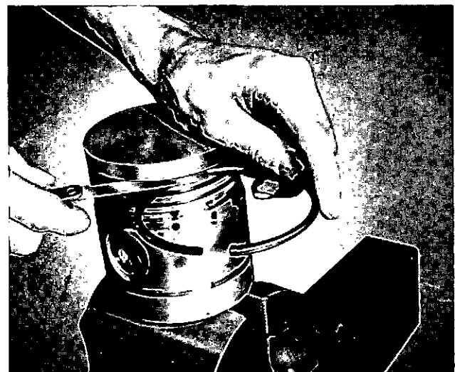
Figure 183—Checking Ring Clearance in Groove
