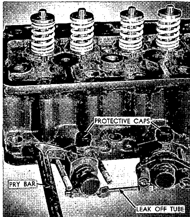
Figure 102 Removing Nozzle Holder Assembly
