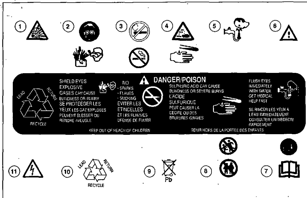
Fig. 1—Typical Battery Labelling
