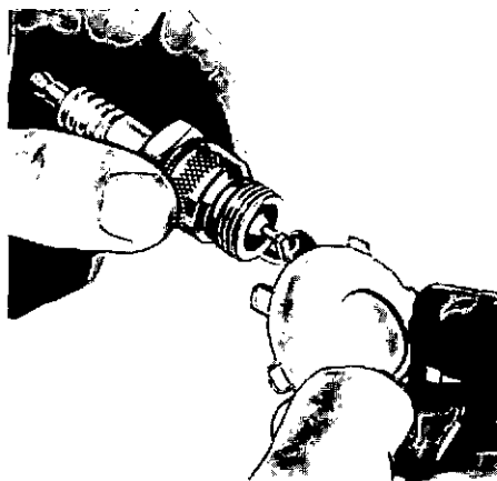
Spark Plug Gapping
