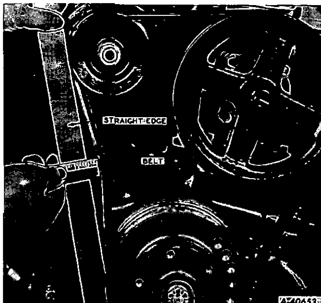
Fig. 12 Checking Belt Tension
