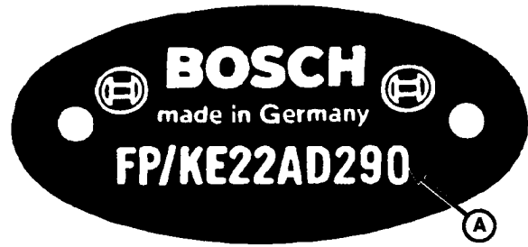
Fuel Supply Pump ID Number
