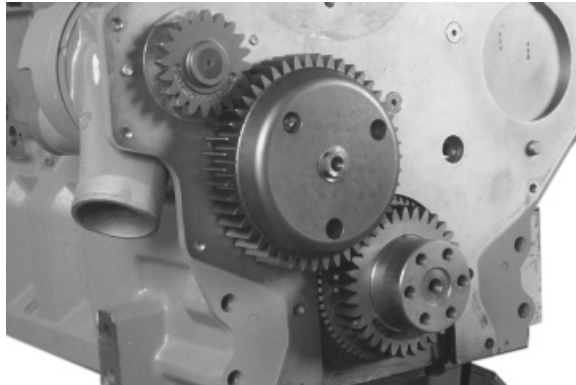
Installing Oil Pump Drive Gear
