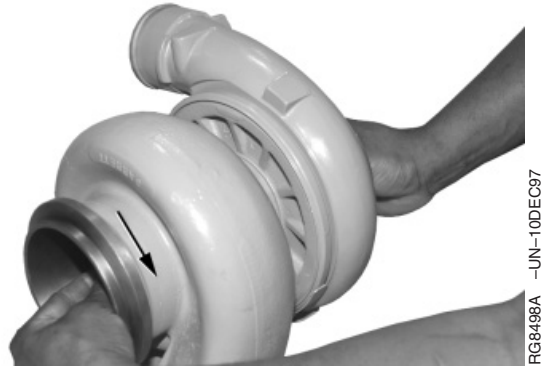
Checking Shaft Rotation and Clearance
