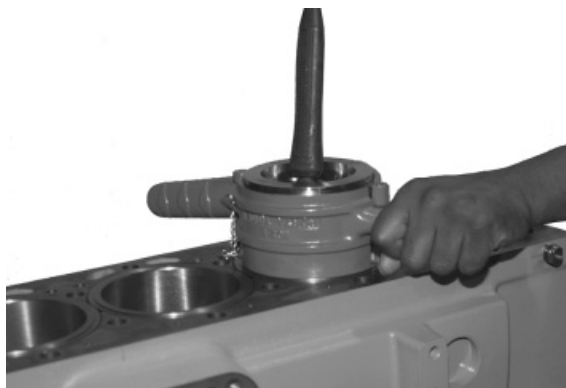
Installing Piston and Rod Assembly
