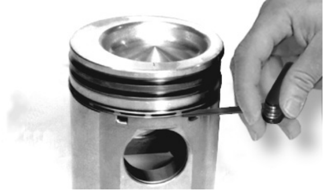
Measuring Oil Control Ring Groove Wear
