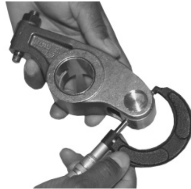
Measure Rocker Arm Roller
