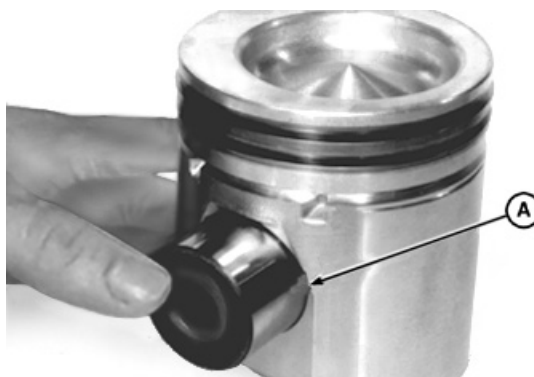
Installing Piston Pin
