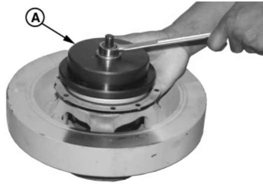
Seating Front Seal on Damper
