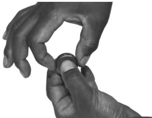
Inspecting Valve Rotator
