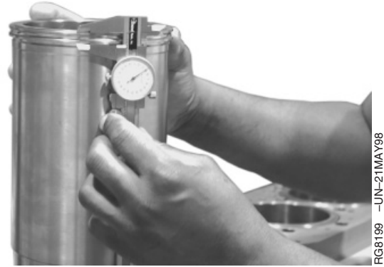
Measuring Liner Flange Thickness
