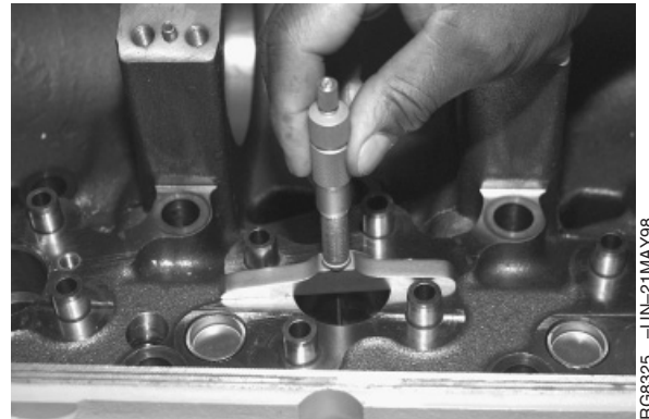
Measuring Cylinder Head Thickness
