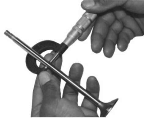
Measuring Valve Stem
