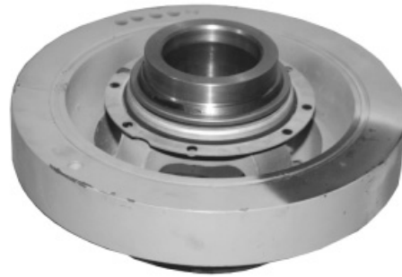
Front Seal Installed on Damper
