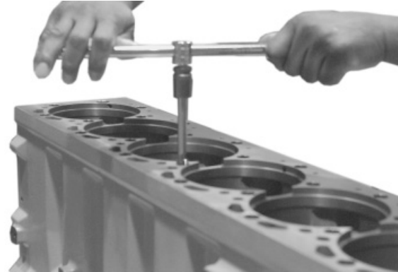
Cleaning Head Bolt Threads in Block
