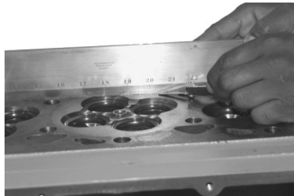
Measuring Cylinder Head Flatness
