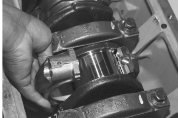
Installing Rod Caps
