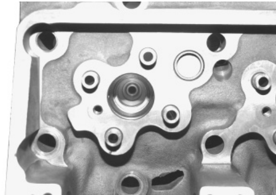
Installed Injector Sleeve
