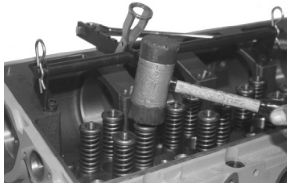
Seating Valve Retainer Locks
