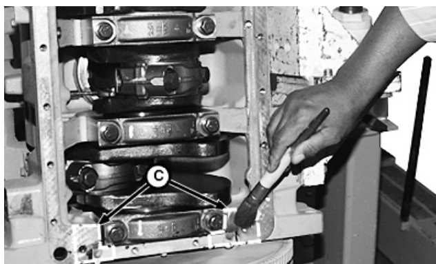
Sealant Applications—Rear Rail
