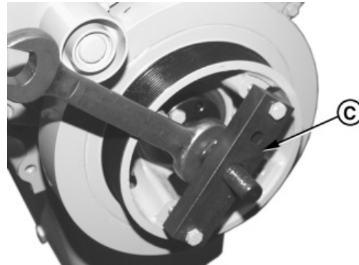
Removing Vibration Damper
