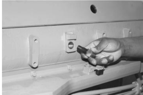
Camshaft Position Sensor
