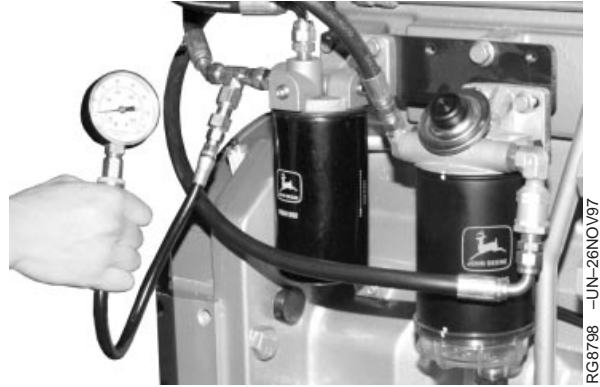
Measuring Fuel Pressure
