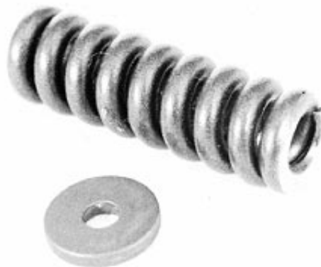
Inspecting Nozzle Spring and Shims
