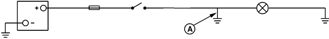
A—Voltage Wire in Contact with Machine Frame
