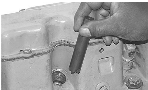
Cleaning Nozzle Seats in Head
