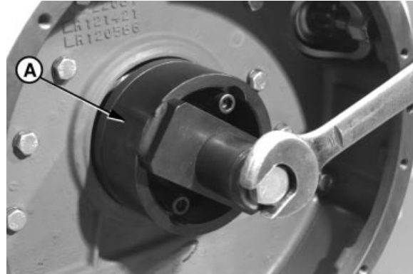
Tightening Guide Plate Cap Screw
