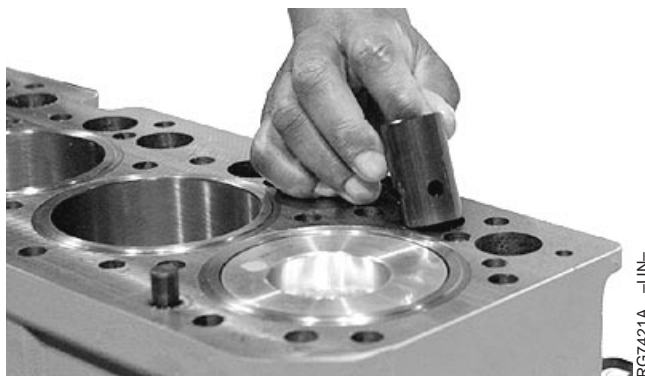
Removing and Cleaning Camshaft Followers
