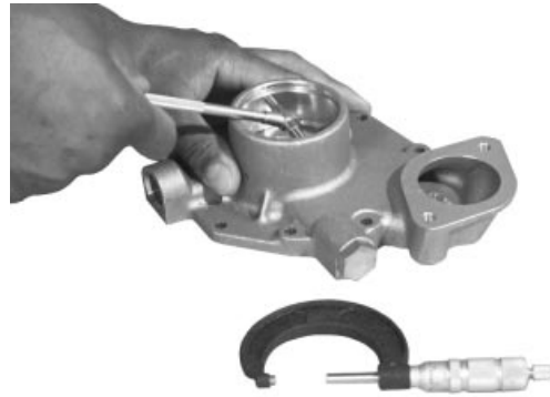
Measuring Impeller Bore
