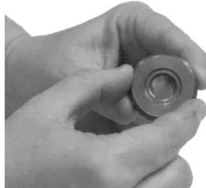
Inspecting Valve Rotators
