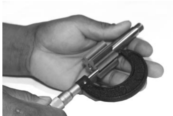
Checking Gear Thickness
