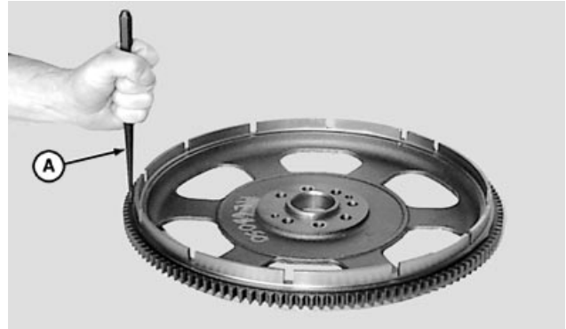
Drive Ring Gear Off Flywheel
