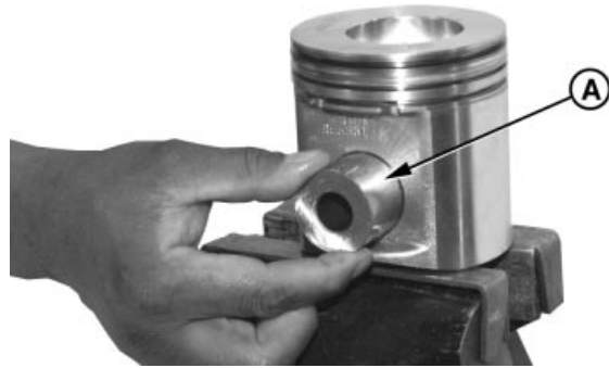
Installing Piston Pin
