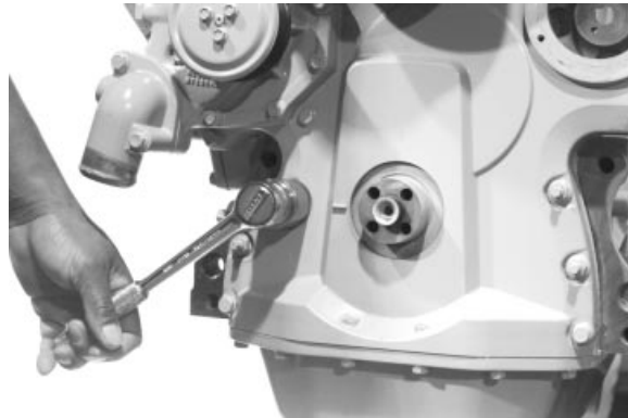
Installing Valve, Spring, Washer, and Plug
