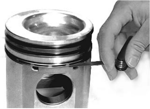
Measuring Clearance with Feeler Gauge
