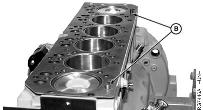
Installing Guide Studs
