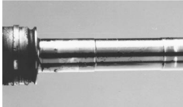
Check for Oil "Coking" on Shaft
