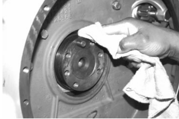
Cleaning Crankshaft Flange
