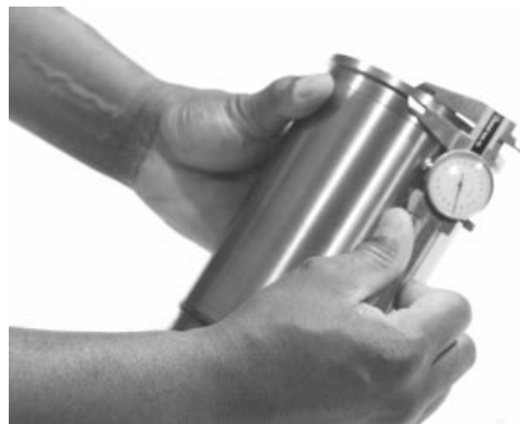
Measuring Liner Flange Thickness
