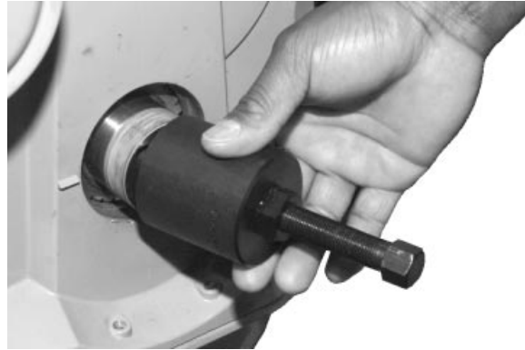
Installing Collet on Crankshaft
