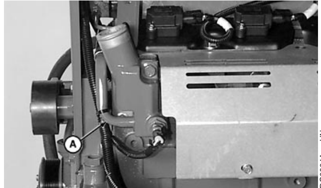
Removing Water Pump Tube
