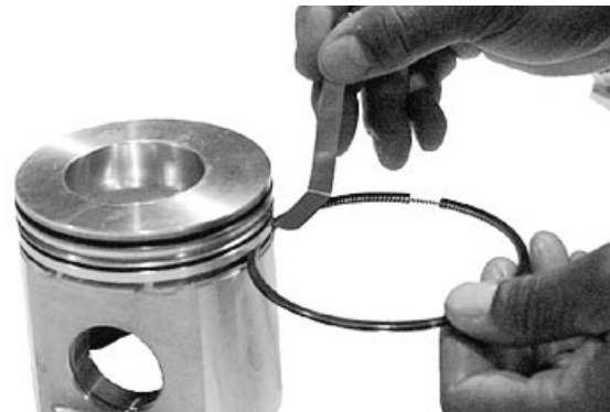
Measure Piston Ring-to-Groove Clearance
