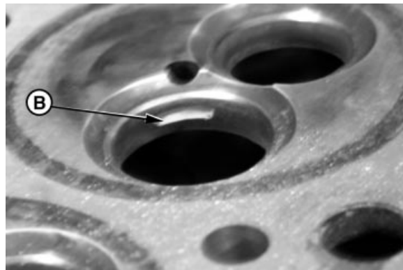
Raising a Burr on Valve Seat
