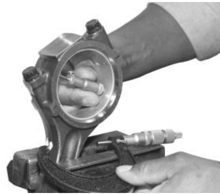
Measuring Connecting Rod
