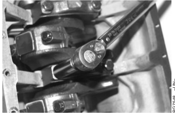
Torquing Main Bearing Caps
