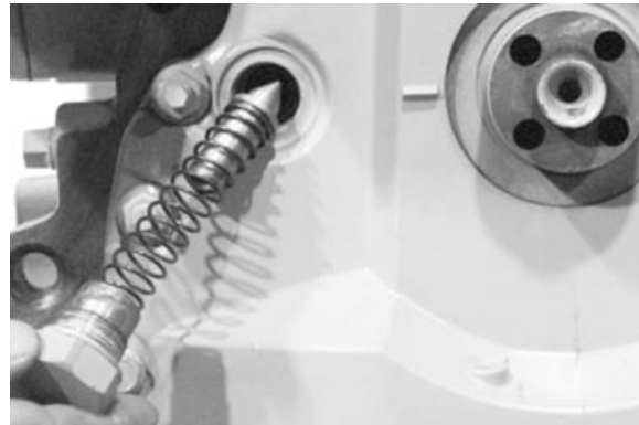
Removing Spring and Valve
