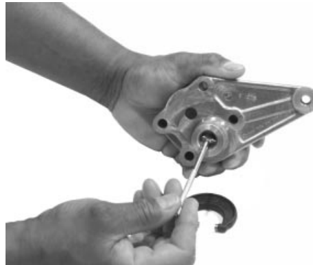
Checking Bushing ID
