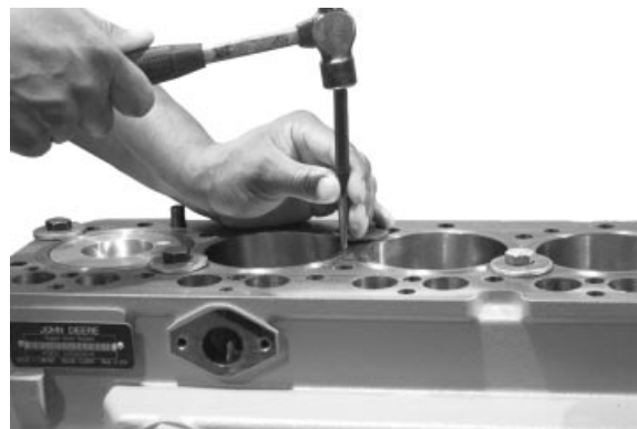
Number Cylinder Liners and Pistons
