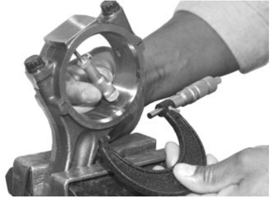
Measuring Rod Bore
