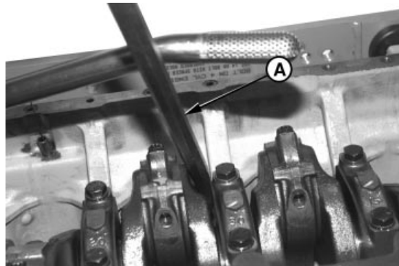
Moving Crankshaft With Pry Bar
