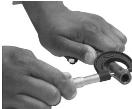
Measure Rocker Arm Shaft OD
