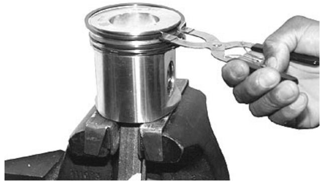
Removing Piston Rings
