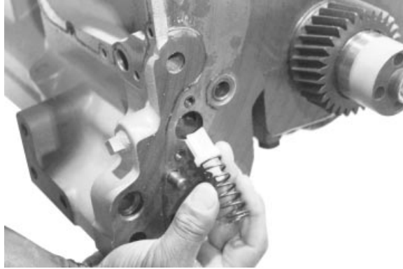
Removing Oil Bypass Valve and Spring
