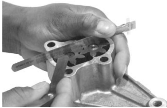
Checking Gear-to-Cover Axial Clearance
