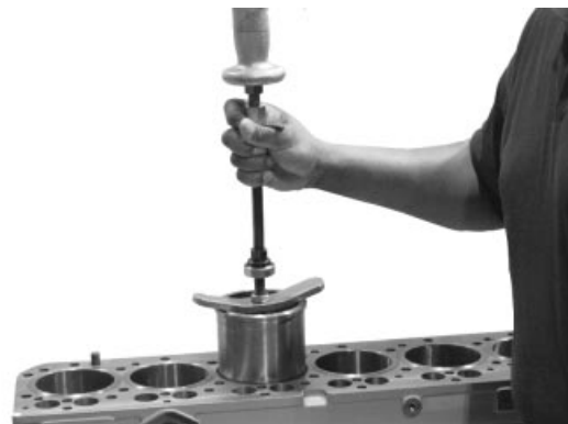
Removing Cylinder Liners
