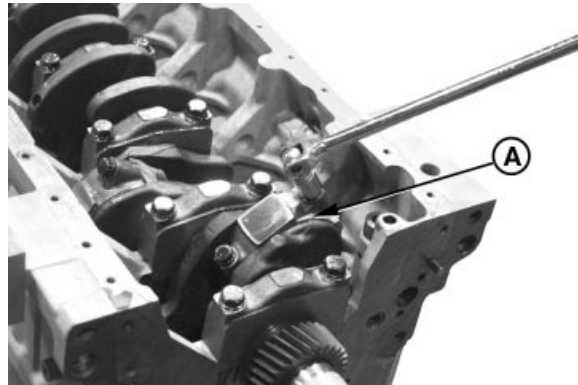
Removing Rod Caps with Bearings
