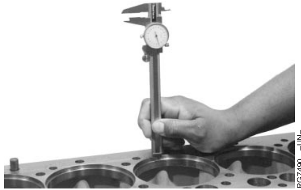
Measuring Liner Flange Counterbore Depth
