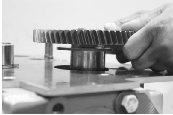
Installing Camshaft Gear
