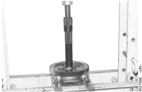
Pressing Gear Off Camshaft
