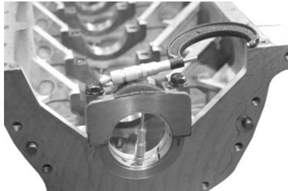
Measure Cylinder Block Main Bearing Bore
