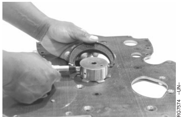
Measuring Shaft OD
