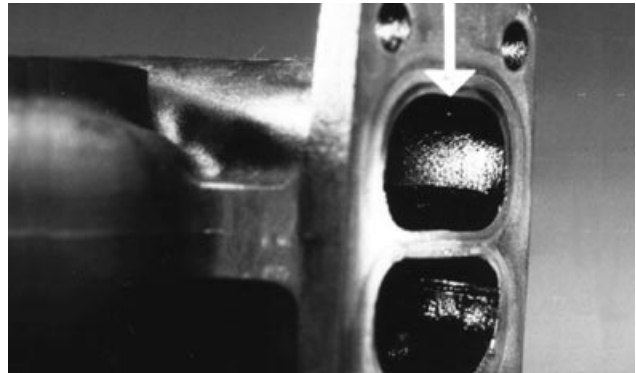
Check Turbine Housing Inlet Ports
