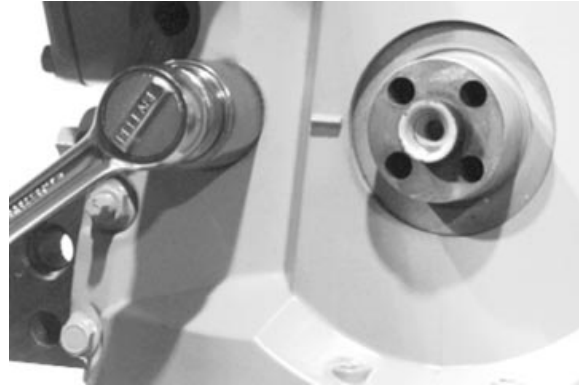
Unscrewing Oil Pressure Regulating Valve Plug
