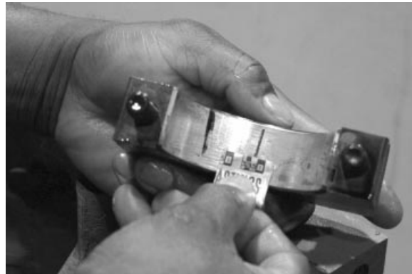
Placing PLASTIGAGE on Bearing Cap
