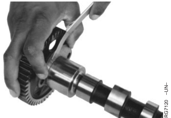
Measuring Camshaft Thrust Plate Clearance
