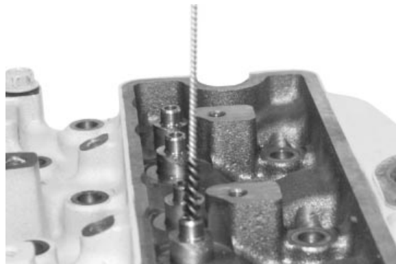
Cleaning Valve Guides
