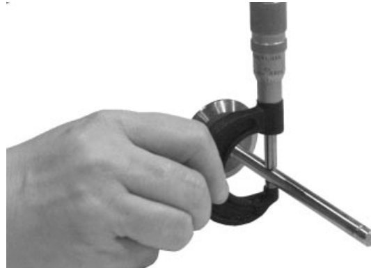
Measuring Valve Guide OD
