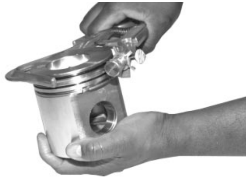
Cleaning Piston Ring Grooves
