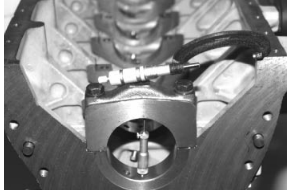
Measuring Bearing Cap Bore ID
