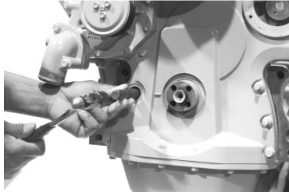
Driving Valve Seat Into Block
