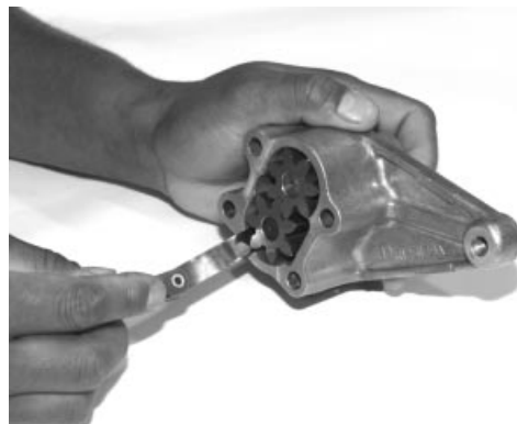
Checking Gear-to-Housing Radial Clearance
