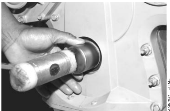
Installing Wear Sleeve
