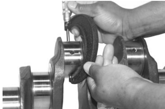
Measuring Crankshaft Rod Journal
