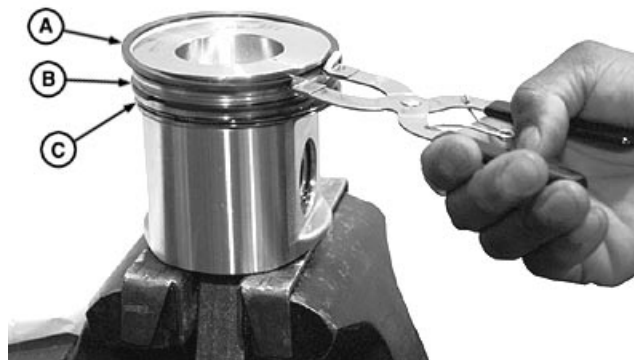
Installing Piston Rings
