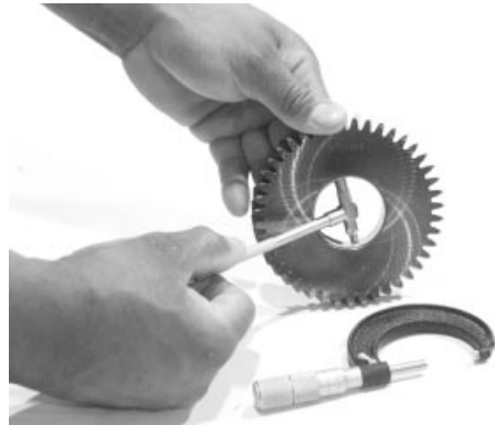
Measuring Idler Gear Bushing ID
