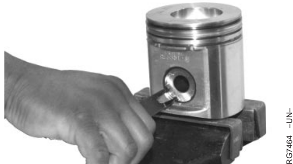
Removing Piston Snap Rings
