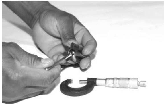
Measuring Idler Gear ID
