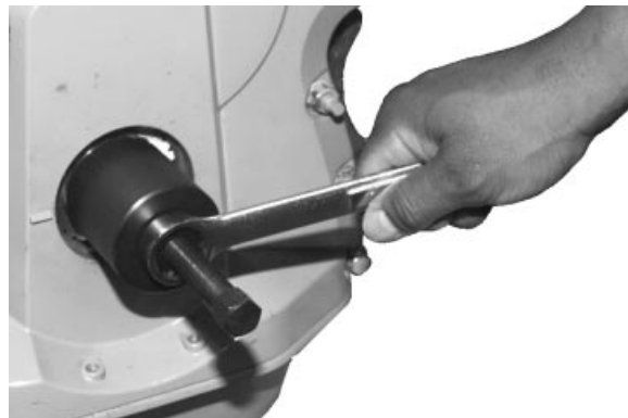
Tightening Forcing Screw
