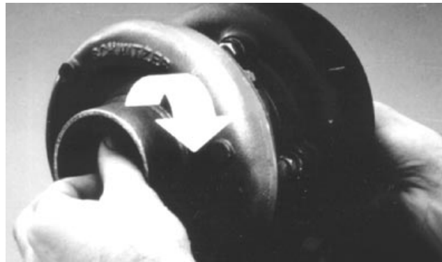
Check Shaft Rotation and Clearance
