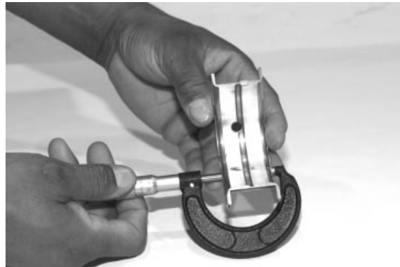
Measuring Thrust Bearing Width
