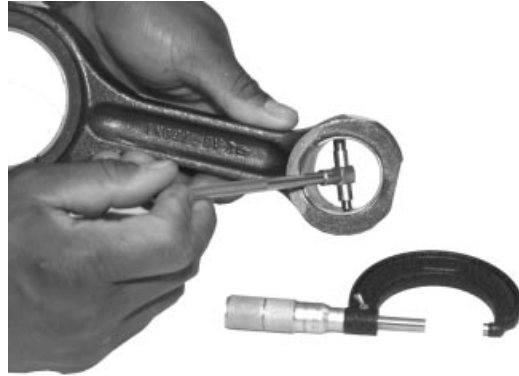
Measuring Pin Bushing ID
