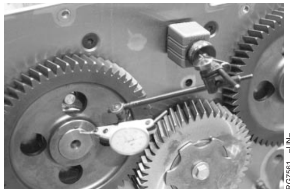
Measuring Camshaft End Play
