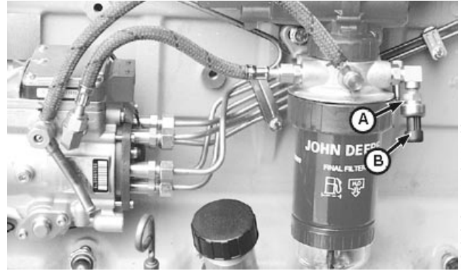
Replace Fuel Pressure Sensor - Tier 1
