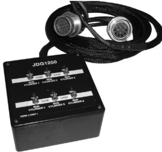
JDG1250 Injector Disable Box
