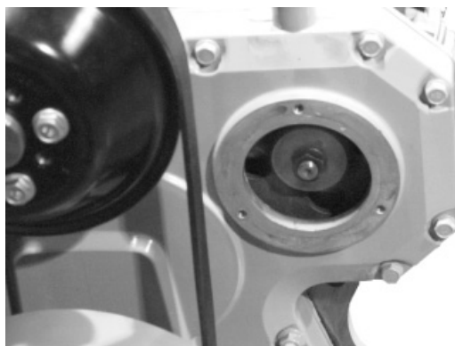
Injection Pump Drive—Cover Removed
