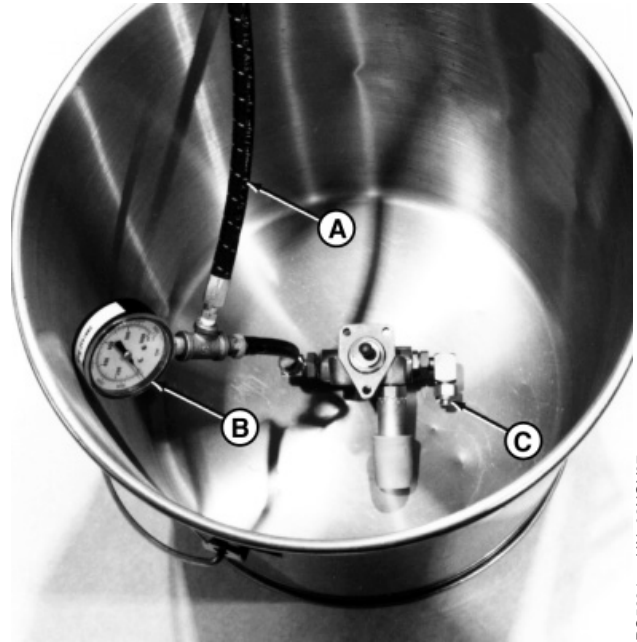
Fuel Supply Pump Leak Test
