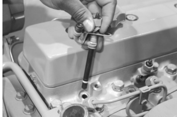
Injection Nozzle in Cylinder Head
