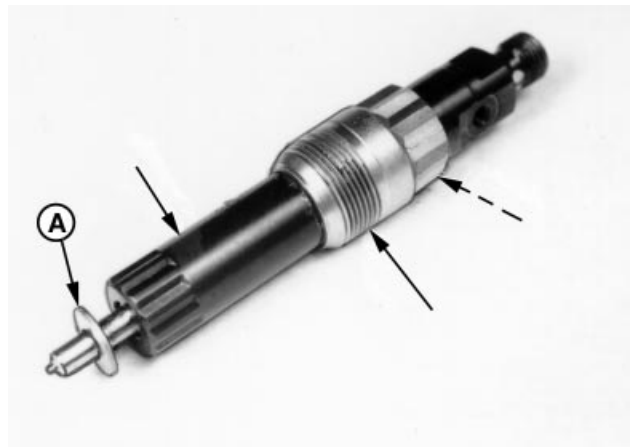
Preparing Nozzle for Installation
