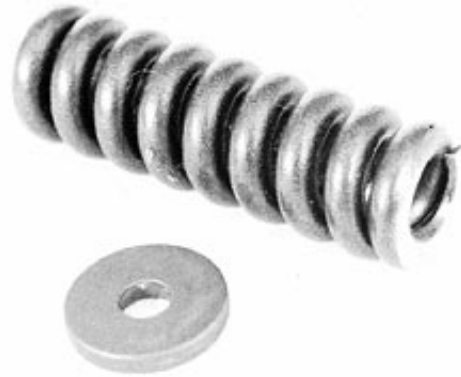
Inspecting Nozzle Spring and Shims
