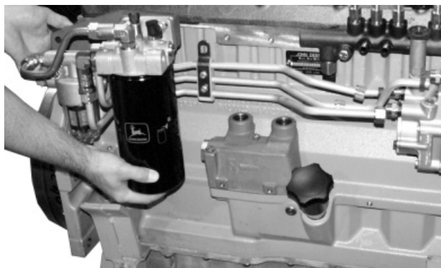
Remove Fuel Filter Assembly (—246269)
