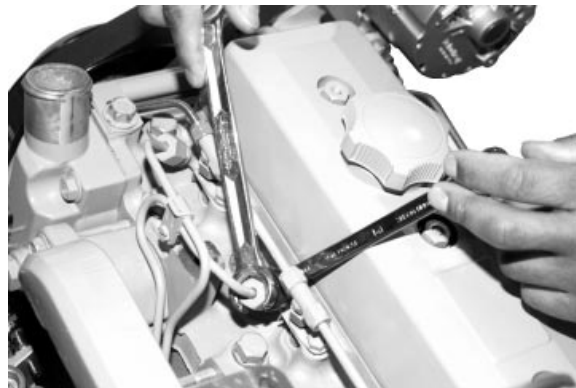
Nozzle Fuel Pressure Line
