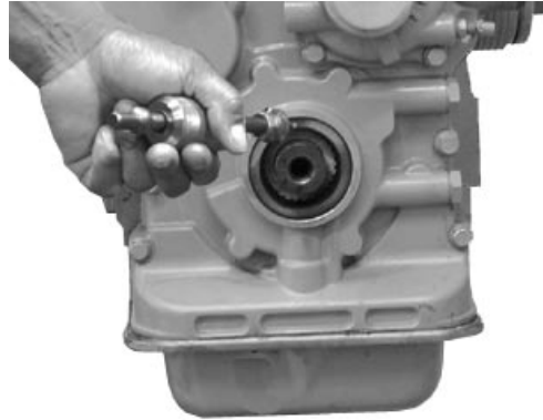
Slide Hammer Installed in Oil Seal
