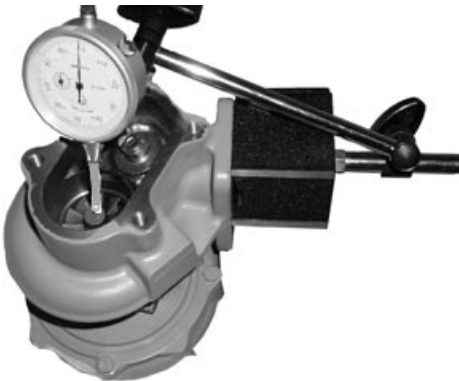
Checking Axial Bearing End Play
