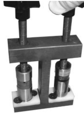
JDG1678 Hydraulic Lifter Bleed-Down Tool
