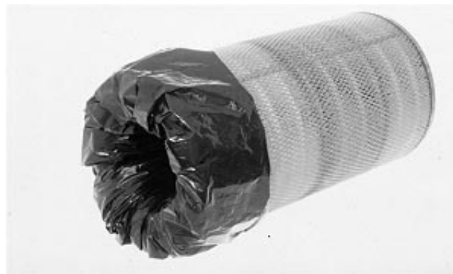
Air Intake Leak Test
