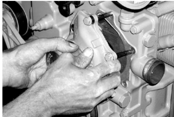
Install Coolant Pump
