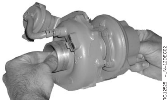
Checking Shaft Rotation and Clearance
