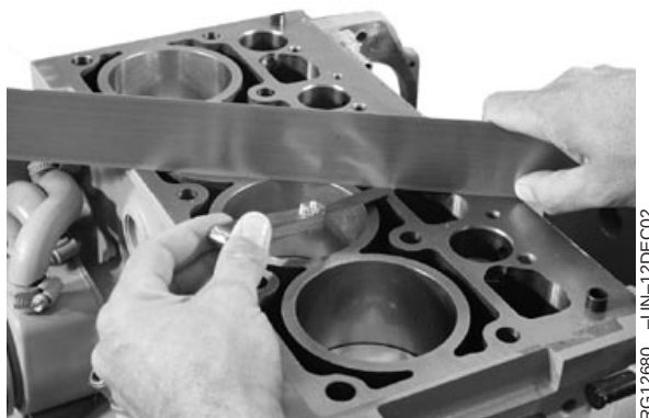
Measuring Cylinder Block Top Deck Flatness
