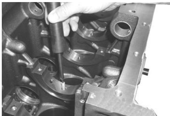
Installing Piston Cooling Orifice
