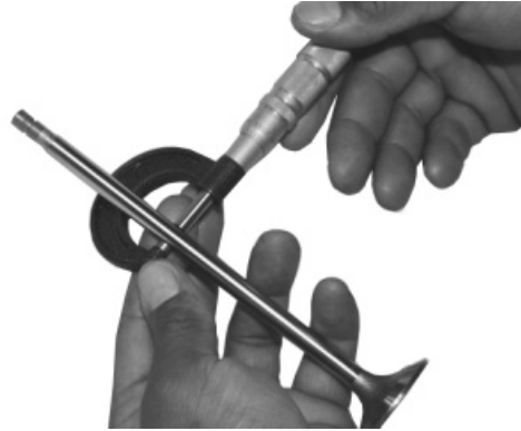
Measuring Valve Stem
