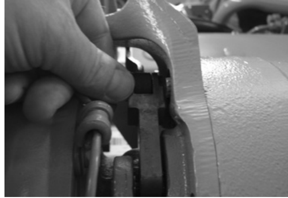
Check for Linkage Free Travel
