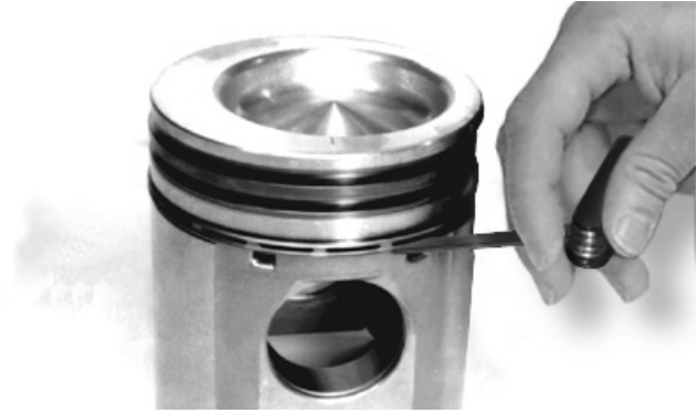
Measuring Oil Control Ring Groove Wear
