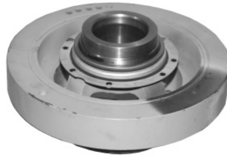
Front Seal Installed on Damper
