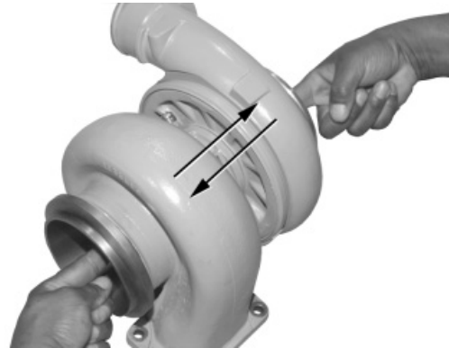
Checking Shaft End Play
