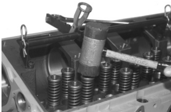
Seating Valve Retainer Locks
