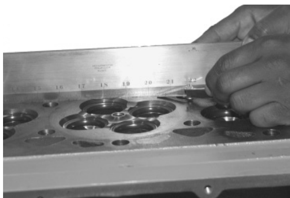
Measuring Cylinder Head Flatness
