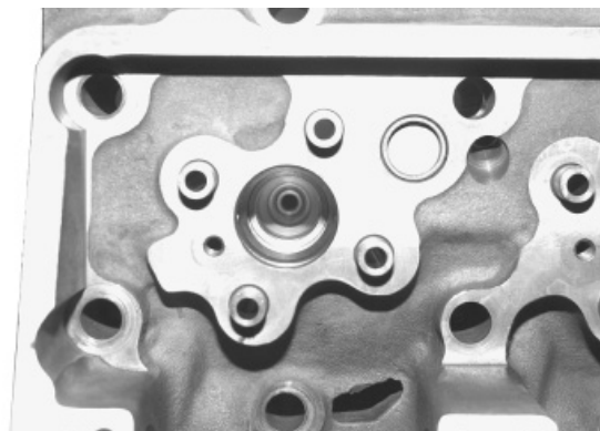
Installed Injector Sleeve
