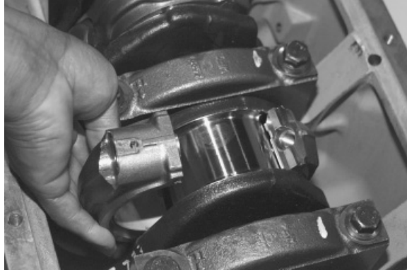
Installing Rod Caps
