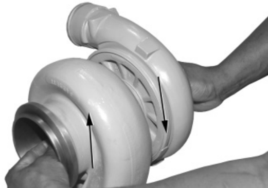
Checking for Contact of Compressor and Turbine Wheels
