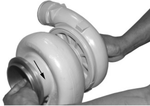
Checking Shaft Rotation and Clearance
