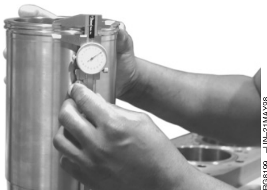
Measuring Liner Flange Thickness
