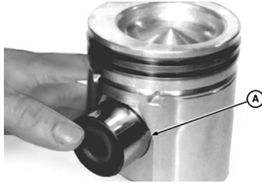
Installing Piston Pin
