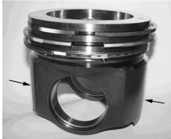
Measuring Piston Skirt
