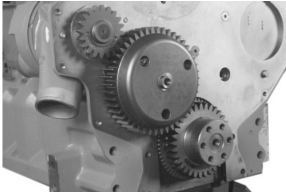
Installing Oil Pump Drive Gear
