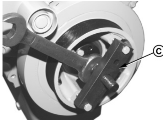
Removing Vibration Damper
