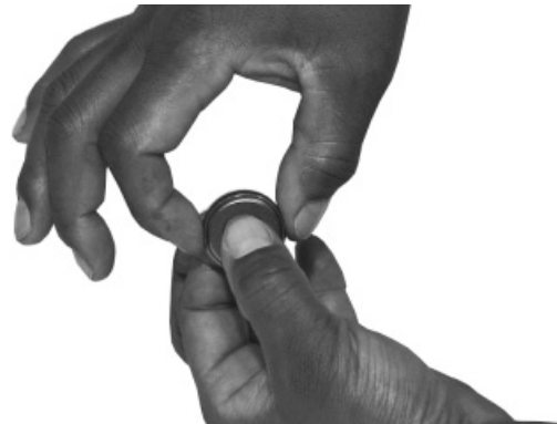
Inspecting Valve Rotator
