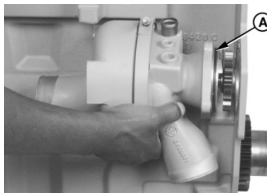
Installing Coolant Pump
