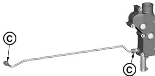
Upper Cylinder Coolant Line
