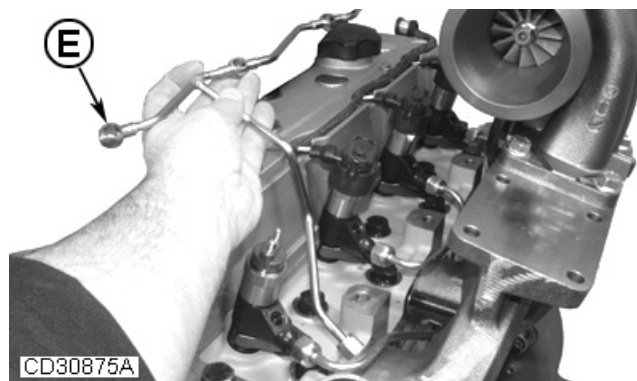
Remove/install fuel leak-off line
