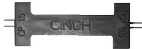
CINCH Terminal Remover Tool
