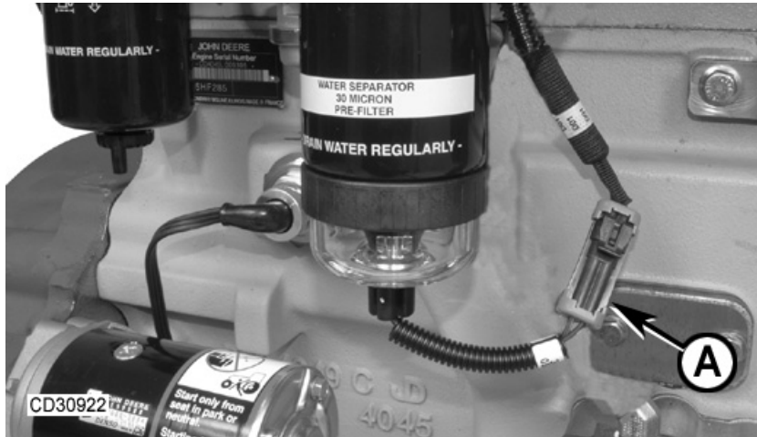
Connect Water-in-Fuel Sensor
