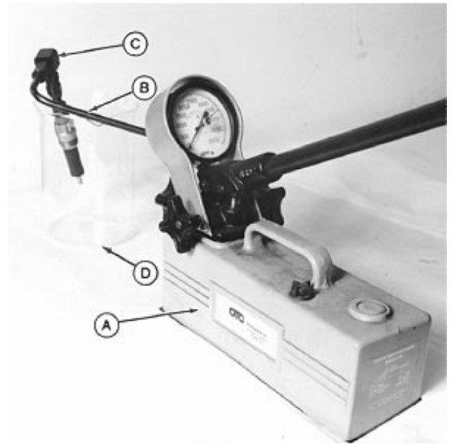
A—Nozzle Tester B—Fuel Line C—Adapter D—Beaker
