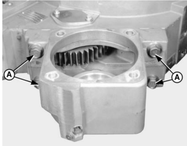
Torque Cap Screws
