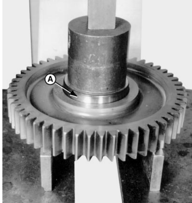
Press on Outer Race of Bearing
