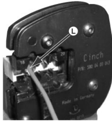
Wire Onto Terminal in Crimping Pliers
