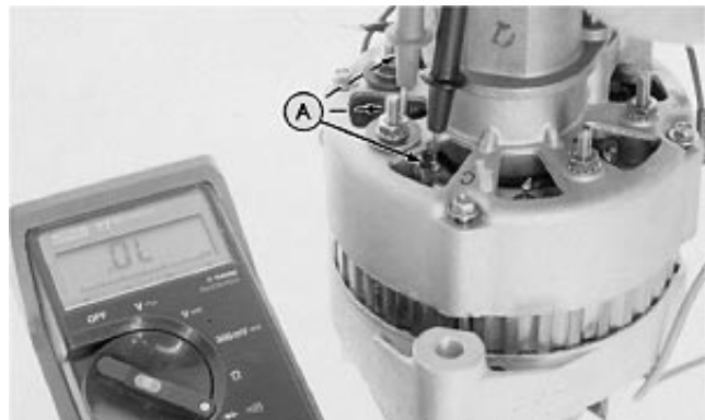
Test Negative Diodes
