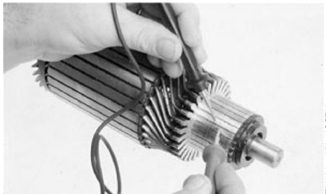
Make Open Circuit Test
