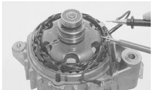
Check Stator and Leads
