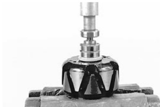
Press Rear Bearing onto Rotor
