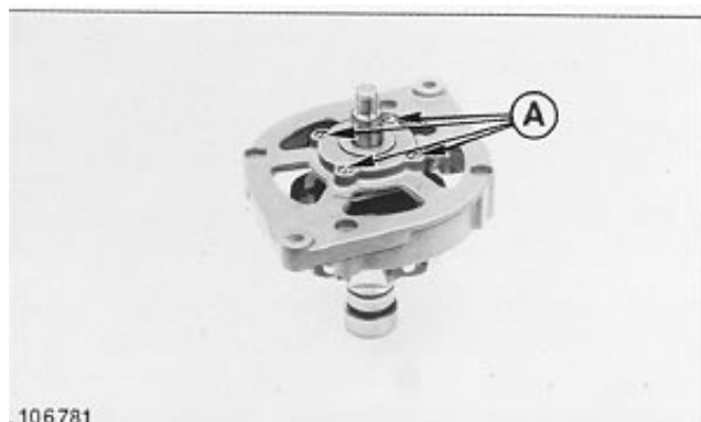
Remove Attaching Screws
