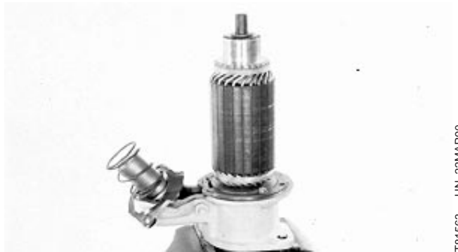
Solenoid Gasket/Plunger Return Spring
