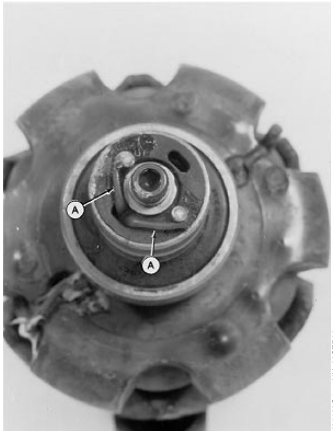
Wrap Leads Around Terminals
