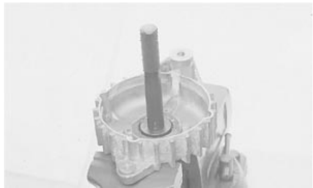
Install Seal in Housing Bore
