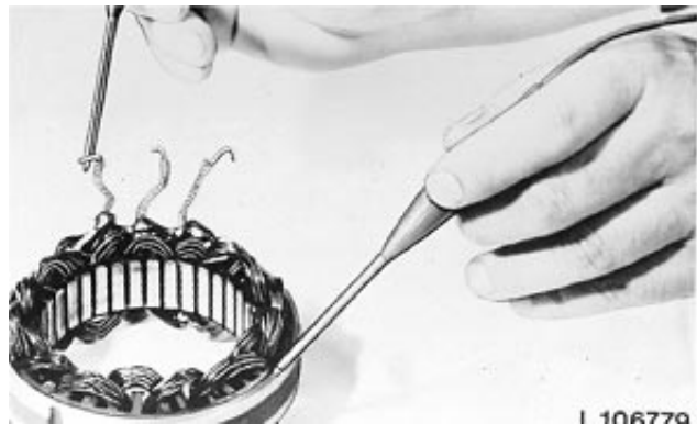
Test Stator Coil for Grounds
