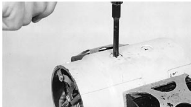
Remove Field Windings
