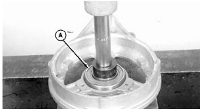
Install Front Ball Bearing
