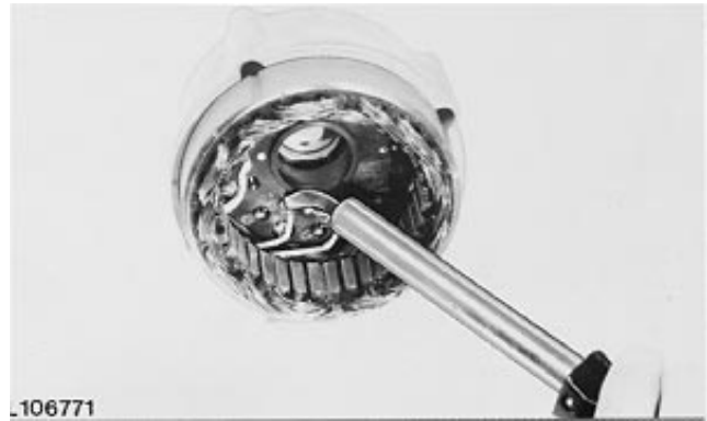
Unsolder Stator Windings
