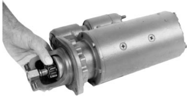
Turn Overrunning Clutch Pinion
