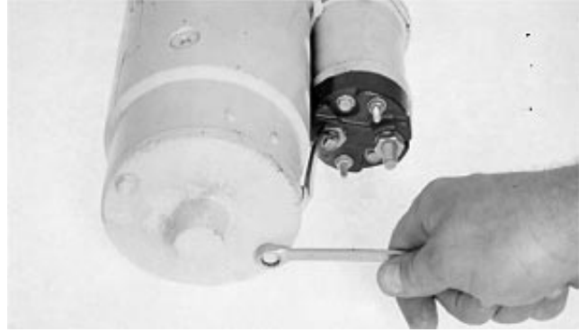
Install Commutator End Frame
