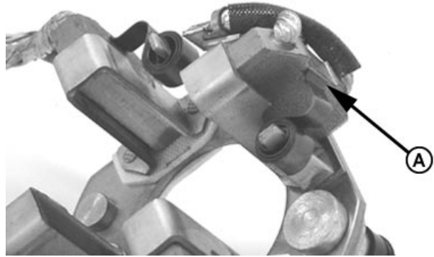
Measure Brush Spring Tension
