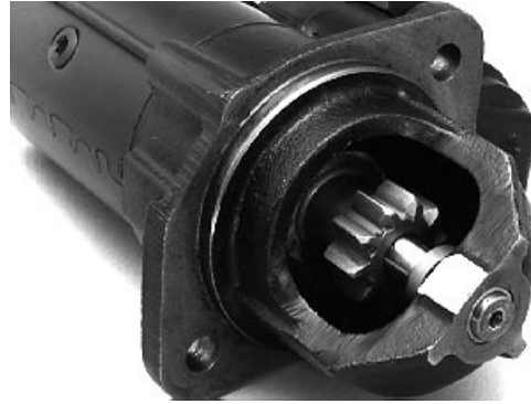
Check Overrunning Clutch Pinion
