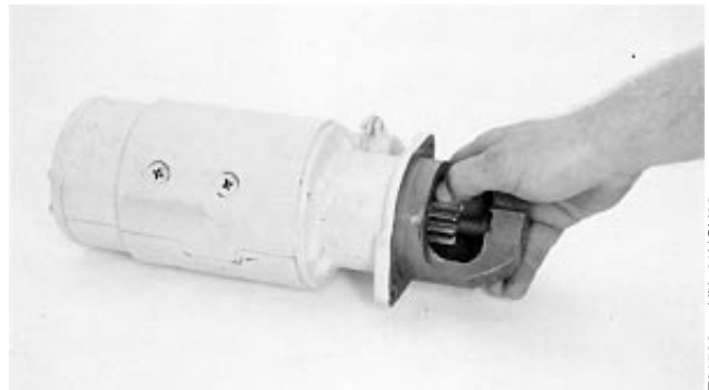
Turn Overrunning Clutch Pinion
