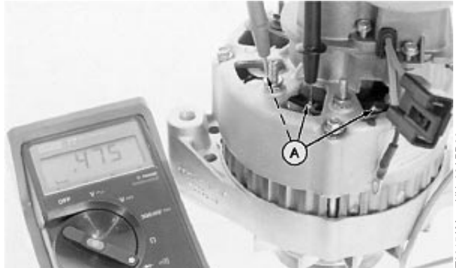
Test Positive Diodes
