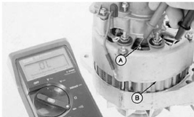
Check Stator for Grounded Winding
