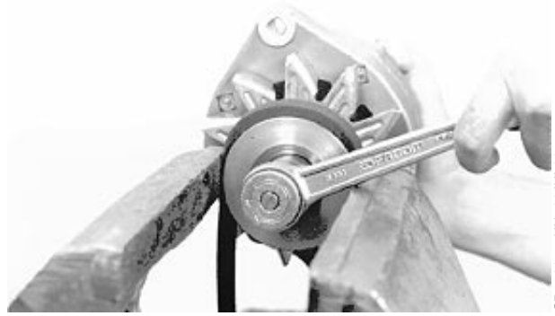
Tighten Pulley Nut
