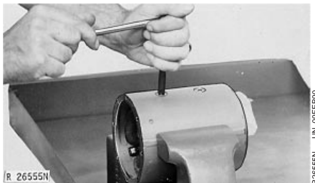
Remove Field Windings
