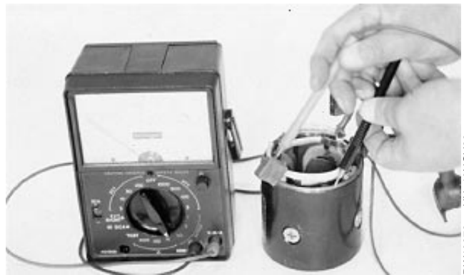
Check for Grounded Field Winding
