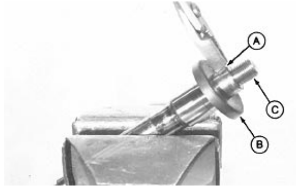
Assemble Roller Bearing Cover
