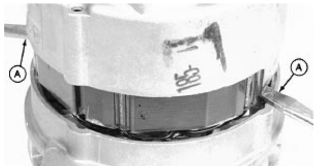
Insert Screwdriver Blades
