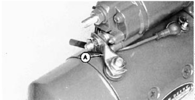
Install Field Coil Connector
