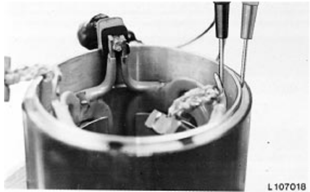
Test Field Winding for Grounded Circuits
