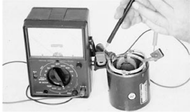
Check for Open Field Coil
