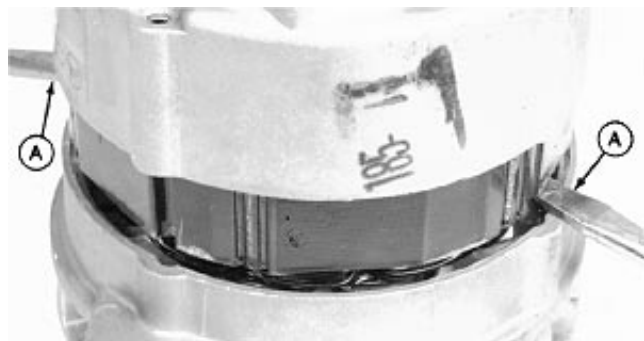
Insert Screwdriver Blades
