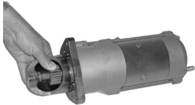
Turn Overrunning Clutch Drive
