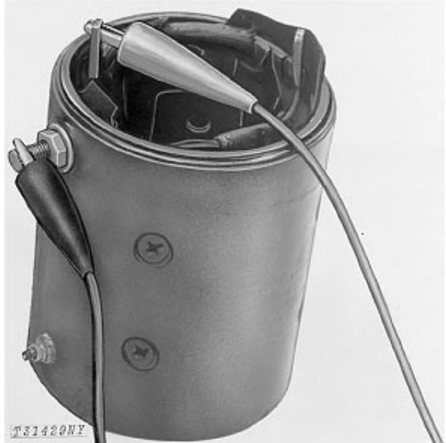
Make Open Circuit Test for Field Windings
