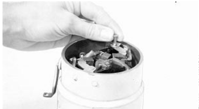
Remove Pins, Holders, and Springs
