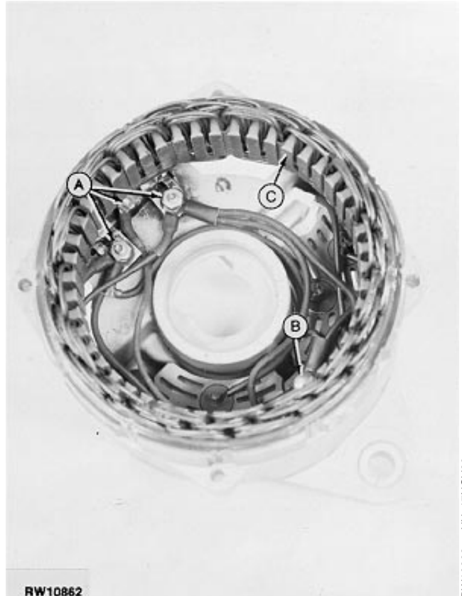
Remove Stator Leads
