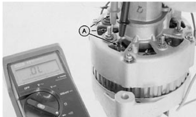
Test Negative Diodes
