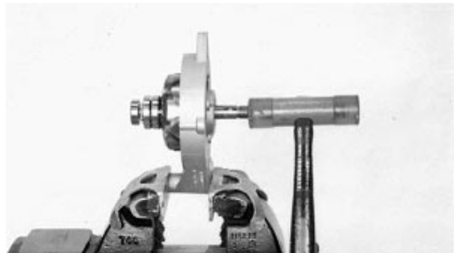
Remove Rotor and Bearing
