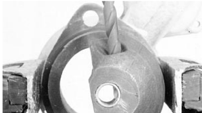
Drive End Wick and Pipe Plug
