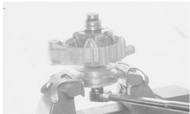
Install Rotor to Housing
