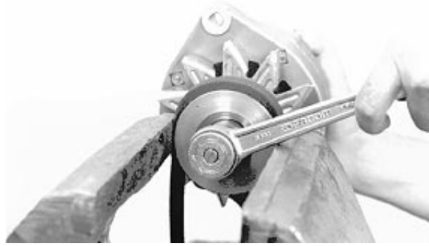
Remove Pulley Nut and Lock Washer
