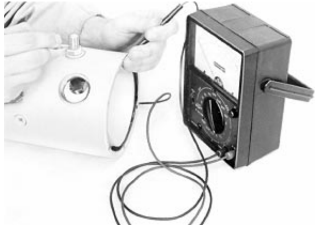
Make Ground Circuit Test
