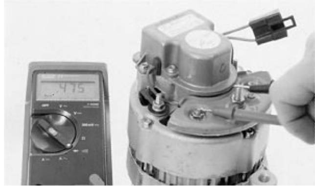
Check Isolation Diode Plate
