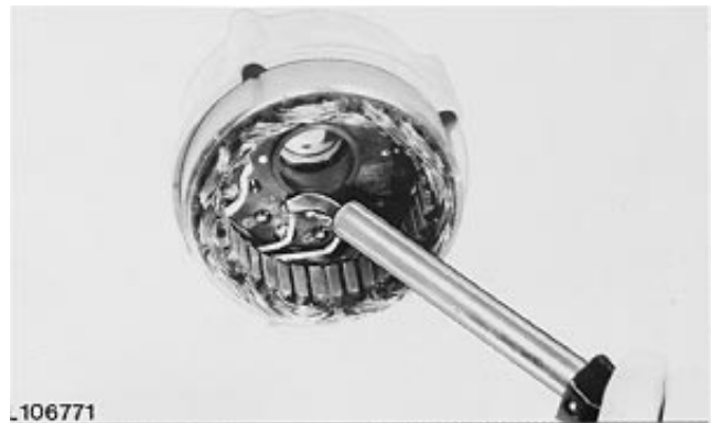
Solder Stator Coils
