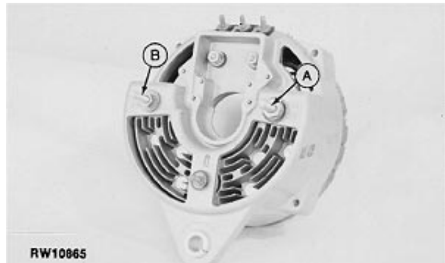
Remove Diode Heat Sink Assembly
