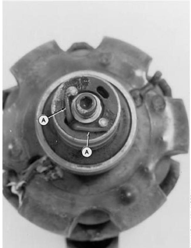
Wrap Leads around Slip Ring Terminals
