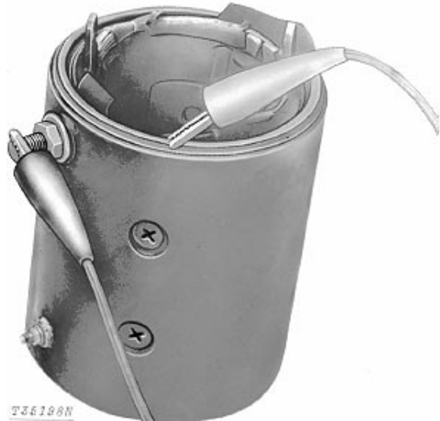
Make Grounded Circuit Test
