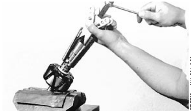
Remove Rear Ball Bearing
