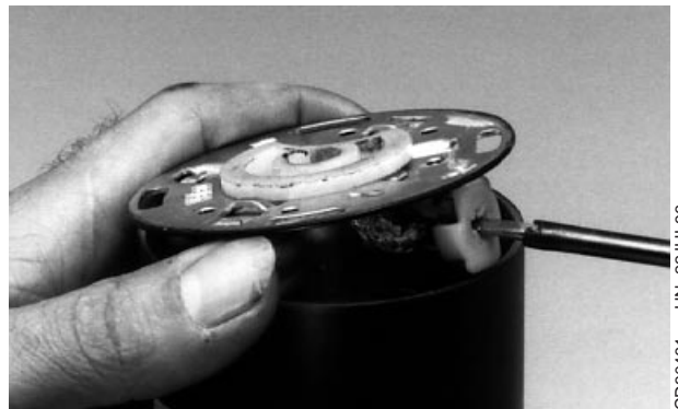
Remove the Disassembly Sleeve
