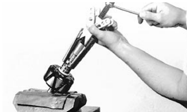
Remove Rear Bearing
