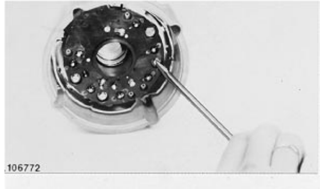
Install Diode Plate
