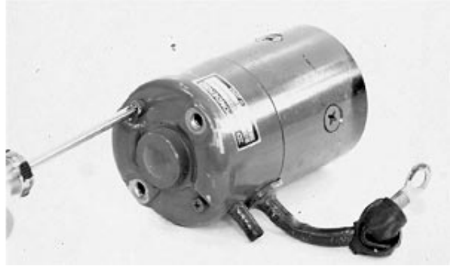
Remove Cap from Frame Assembly
