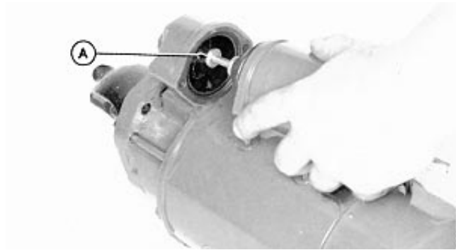
Lift Plunger Shaft
