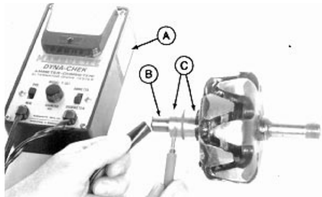
Test Rotor for Grounds
