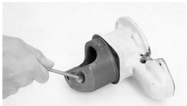
Remove Plug and Drive End Wick
