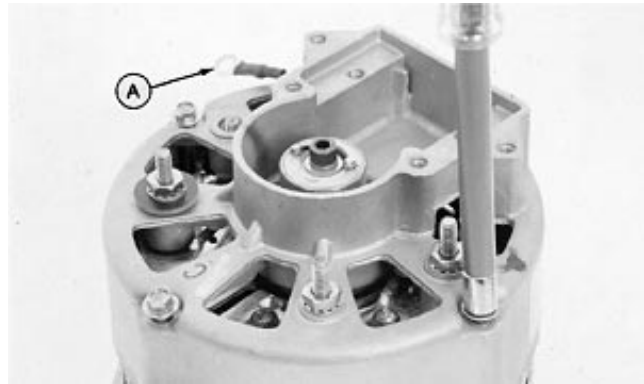
Disconnect Wiring Lead
