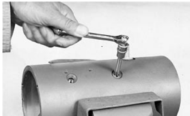
Remove Field Windings
