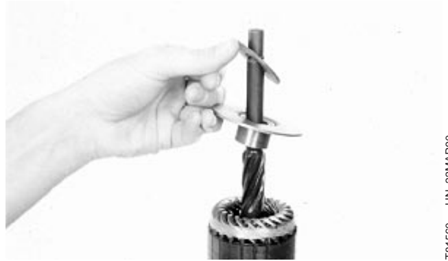
Lubricate Splines and Armature Shaft
