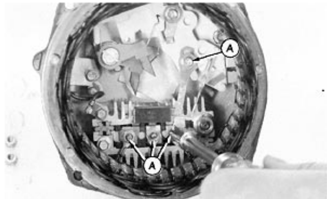
Stator and Diode Trio
