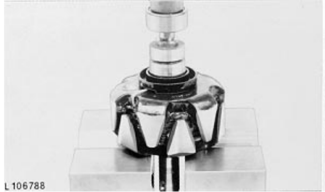
Pressing Ball Bearing Onto Rotor Shaft
