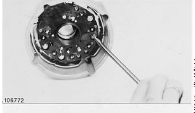
Diode Plate Removal
