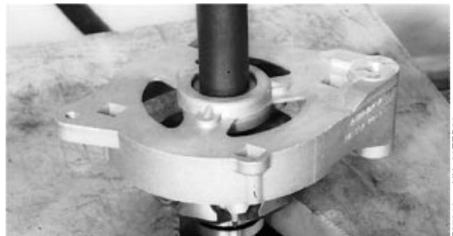
Press Front Housing onto Rotor Shaft
