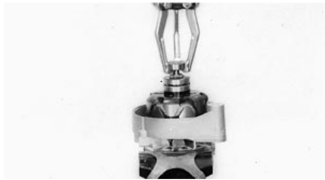
Remove Slip Ring End Bearing
