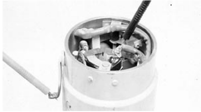
Make Open Circuit Test
