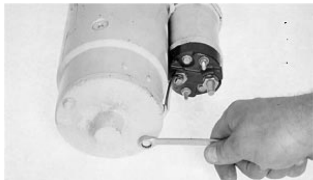
Remove Commutator End Frame
