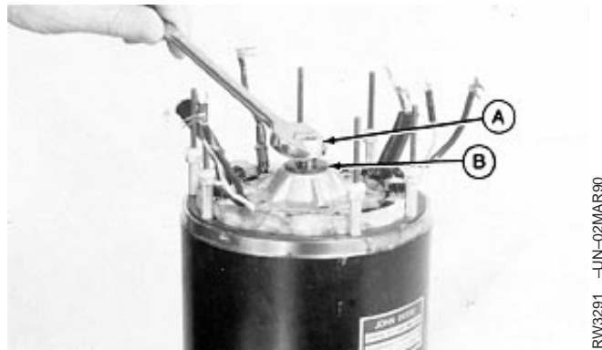
Remove Lock Nut and Washer
