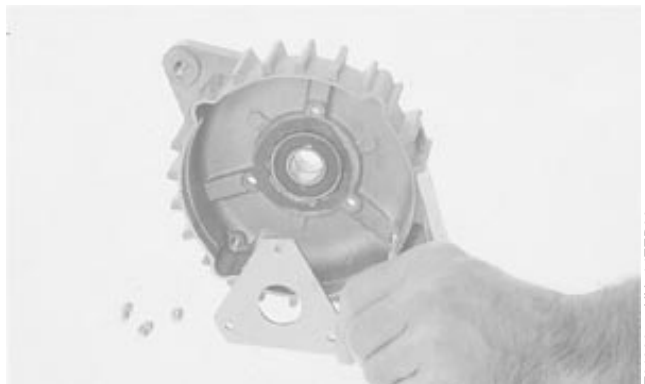
Install Bearing Retainer
