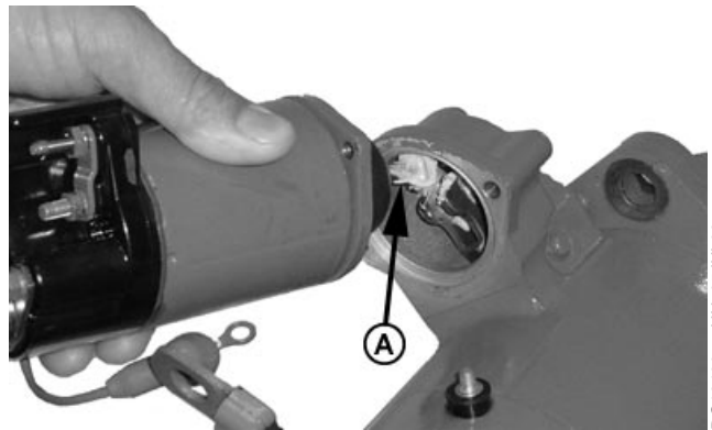
Solenoid Plunger Shaft
