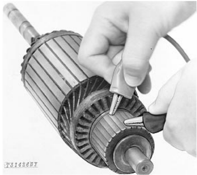
Make Open Circuit Test
