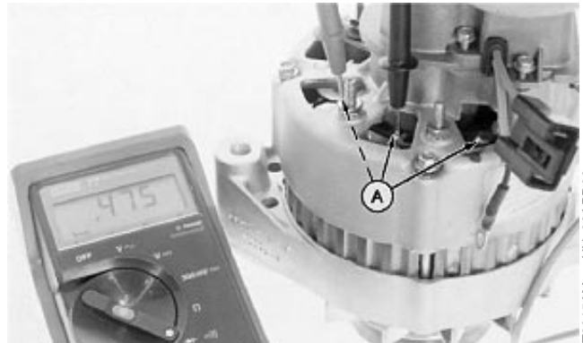
Test Positive Diodes
