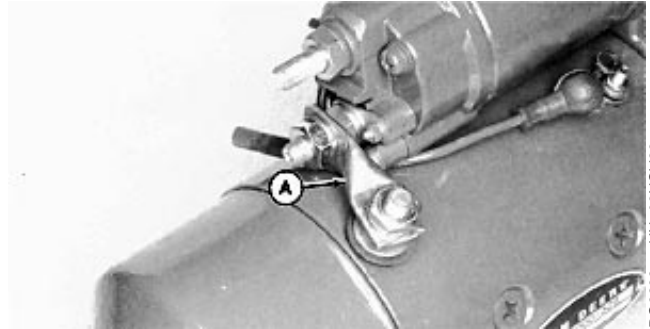
Remove Field Coil Connector
