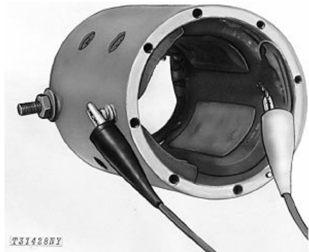
Make Open Circuit Test for Shunt Windings
