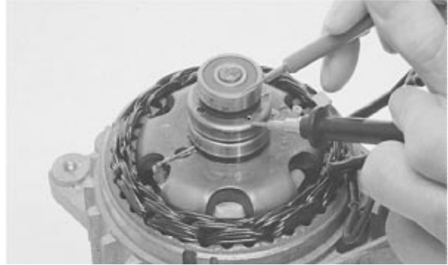
Check for Grounded Rotor Windings
