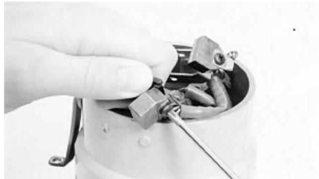
Tighten Screws Securely
