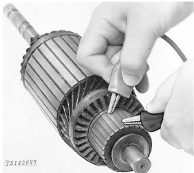
Make Open Circuit Test
