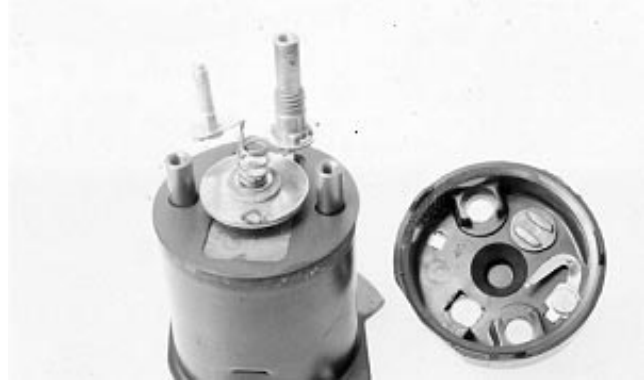
Inspect and Clean Solenoid Parts
