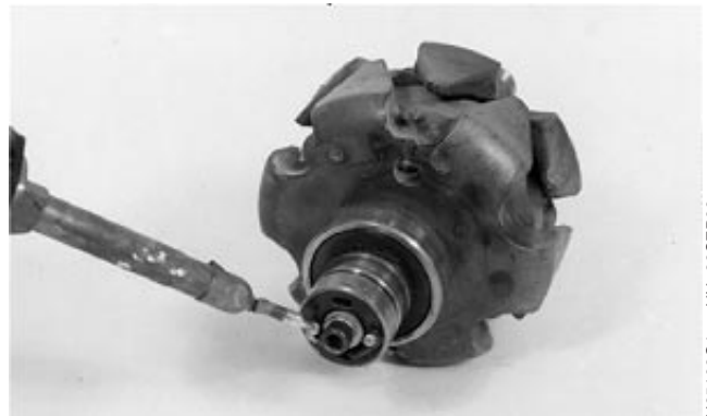
Unsolder Rotor Leads
