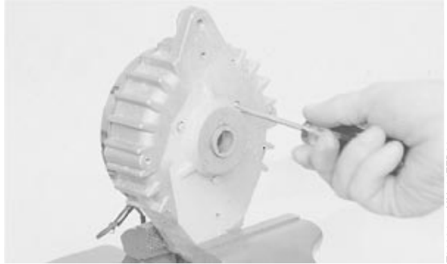
Remove Bearing Retainer
