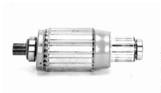
Inspect and Repair Armature
