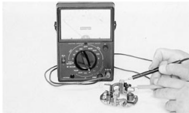
Test Brush Holder with Ohmmeter
