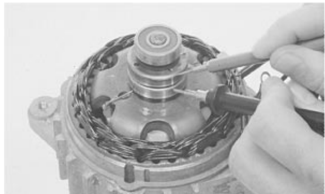
Check Rotor Windings
