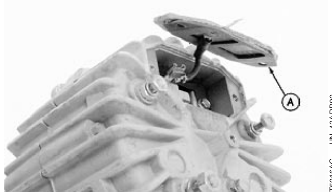
Remove Brush Cover and Gasket
