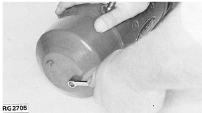
Remove End Frame Cover and Gasket
