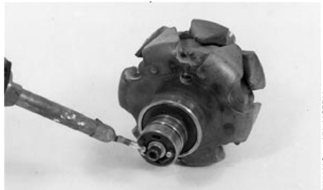
Inspect Rotor Shaft and Body
