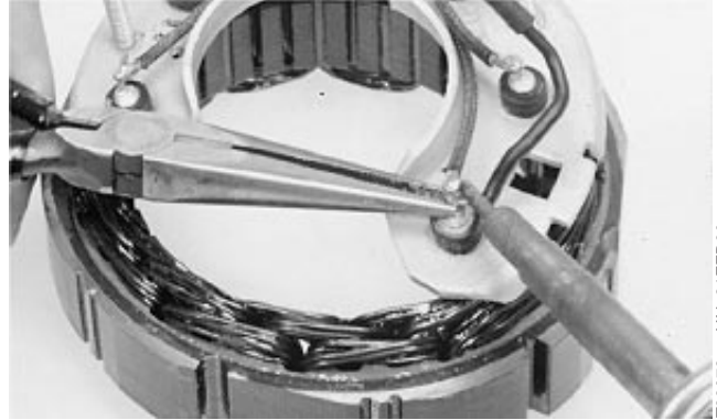
Unsolder Wiring Leads
