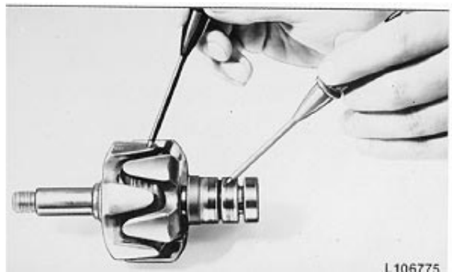
Test Rotor for Ground
