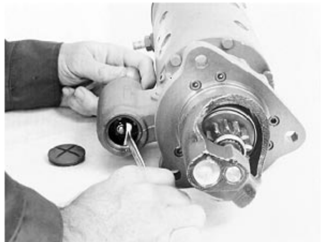
Remove Self-Locking Nut
