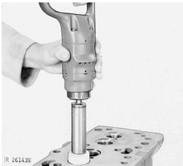
Grinding Valve Seats
