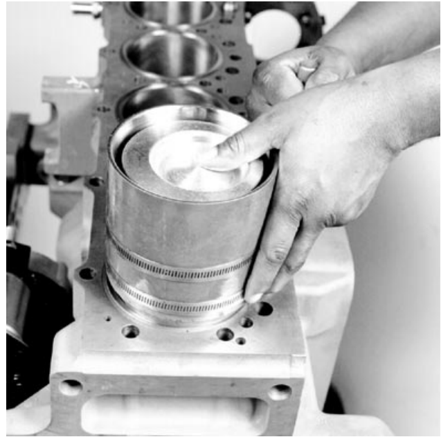
Installing Piston in Cylinder Liners
