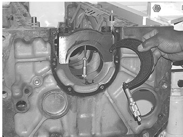
Measuring Main Bearing Cap Bores
