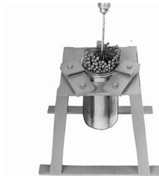
Deglazing Cylinder Liners
