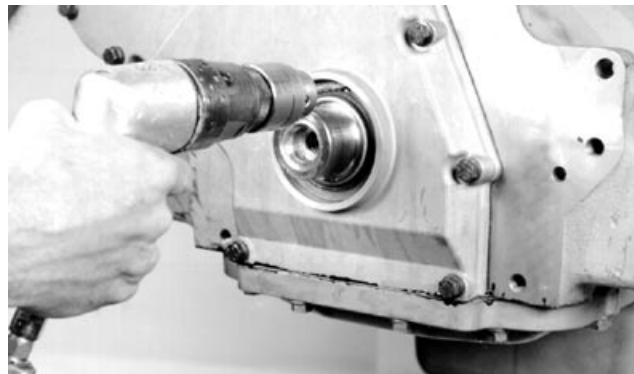
Drilling Hole in Front Oil Seal Casing
