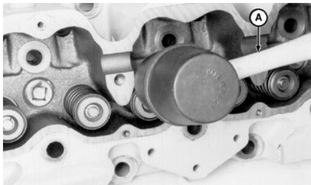
Seating Retainer Locks on Valves
