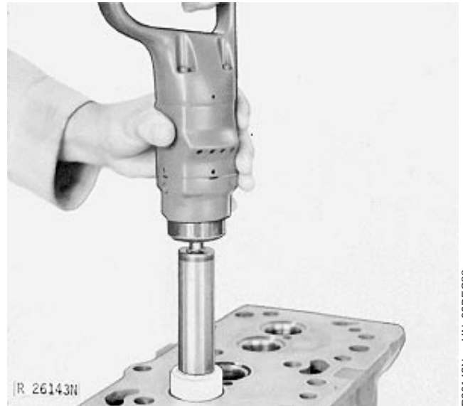
Grinding Valve Seats
