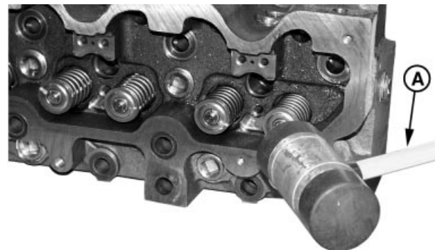
Seating Retainer Locks on Valves
