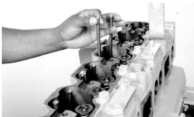
Installing Push Rods and Caps
