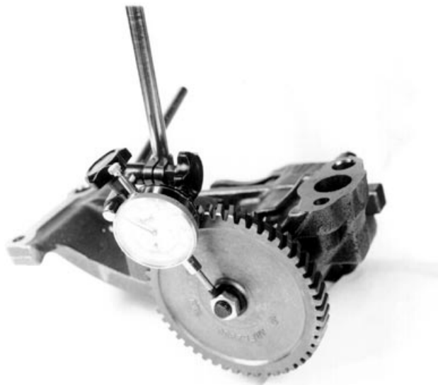
Check Pump Drive Shaft Side Movement
