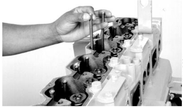
Installing Push Rods
