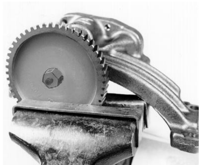
Inspect Oil Pump Drive Gear
