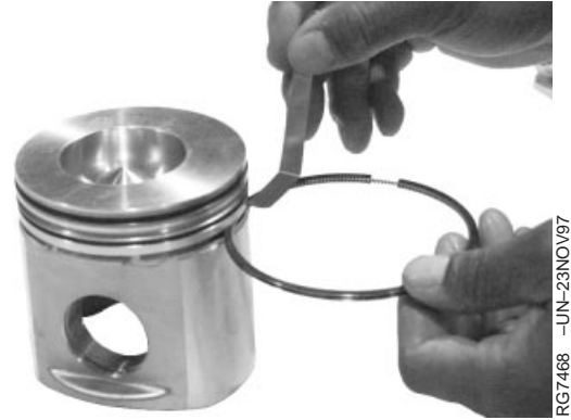
Check Groove Wear
