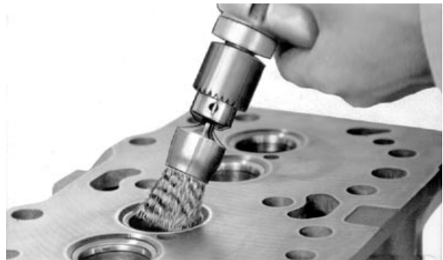
Clean and Inspect Valve Seats
